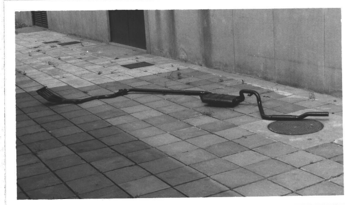
I, silencer + exhaust pipes after exhaust manifold.
