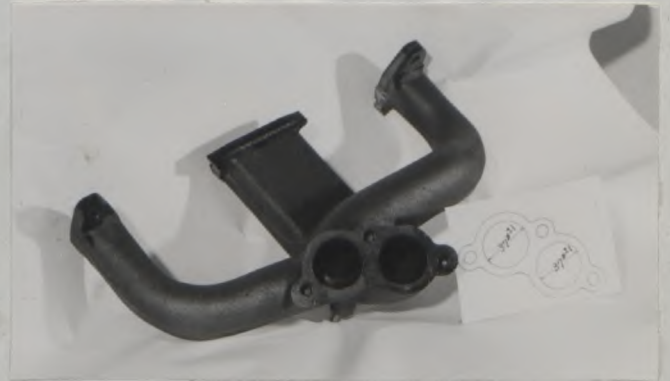
Q, exhaust manifold
