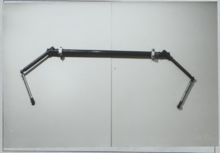
Photo No TU5 Shock absorber cooling tube
