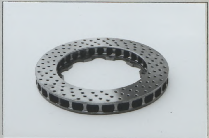
PHOTO No VW6 Front and/or Rear brake discs, TYPE Y
