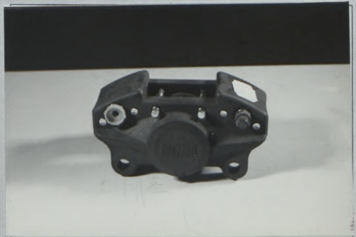
Photo No W3 Rear brake caliper, TYPE O
