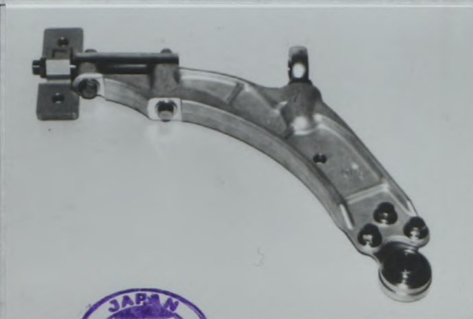
PHOTO No T5 Reinforced transeverse link TYPE A
