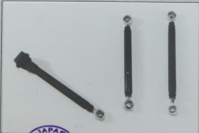
PHOTO No U3 Reinforced rear links TYPE A
