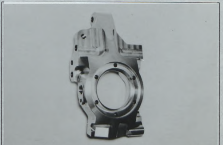
PHOTO No T4 Reinforced front knuckle TYPE D
