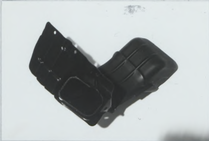
Photo No VW6 Brake cooling duct, TYPE F
