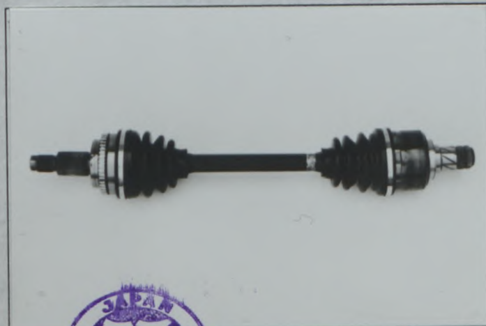
PHOTO No Z5 Reinforced drive shaft front left TYPE B
