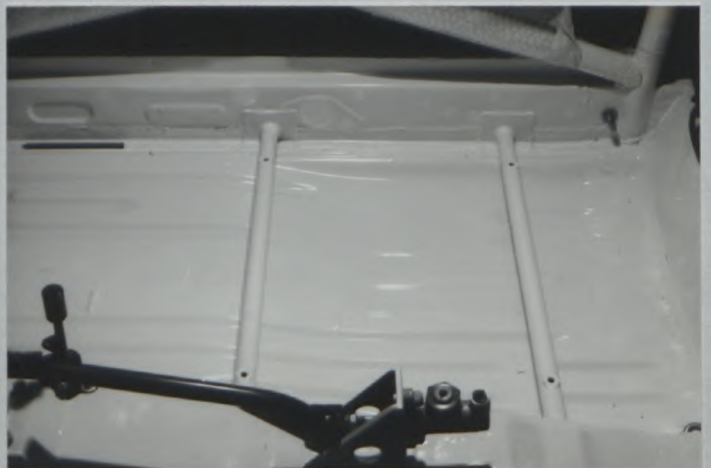
Photo No FF2 Seat anchorage, TYPE E
