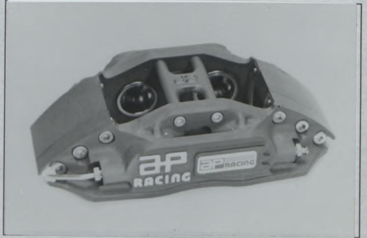
PHOTO No VW4 Brake caliper TYPE F
