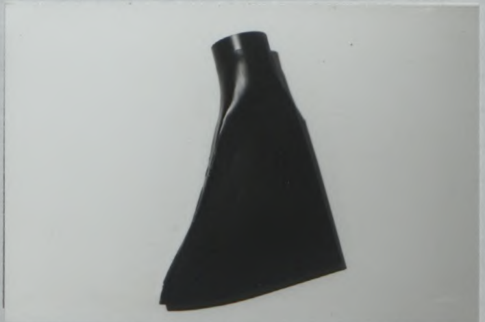
Photo No VW3 Brake cooling duct, TYPE C
