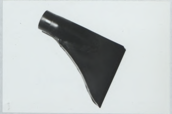
Photo No VW7 Brake cooling duct, TYPE G
