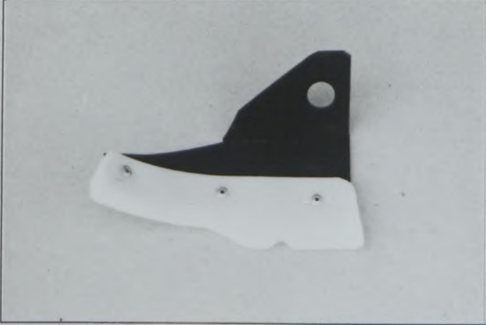
PHOTO No VW14 Front/rear brake scraper TYPE A
