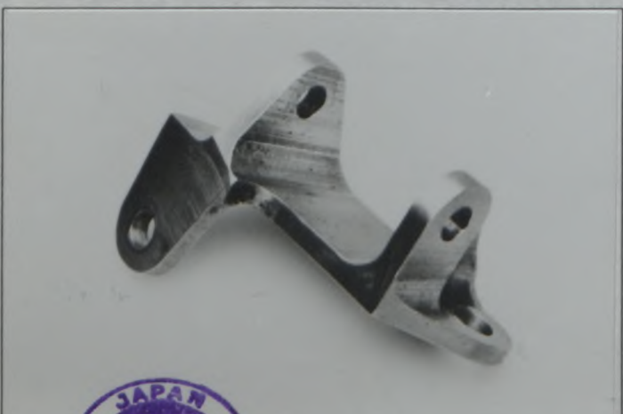
PHOTO No Z30 Heavy duty steering knuckle arm TYPE E
