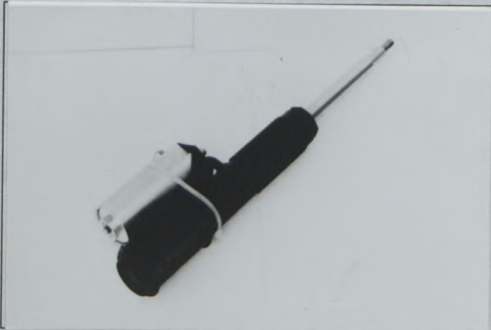
PHOTO No U12 Heavy duty rear strut TYPE E
