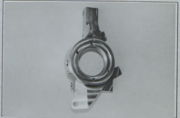
PHOTO No U2 Reinforced rear knuckle TYPE B
