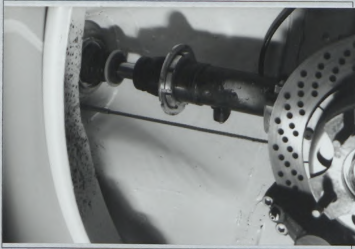
Photo No TU2 Reinforced stabilizer with adjustment linkage optional, TYPE A
