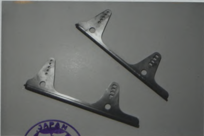
Photo No FF1 Seat supports, TYPE D
