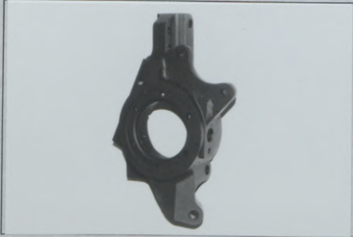
PHOTO No U1 Reinforced rear knuckle TYPE A
