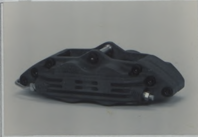
Photo No W2 Rear brake caliper, TYPE N
