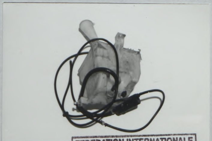
Photo No VW9 Brake & shock absorber cooling reservoir TYPE B
