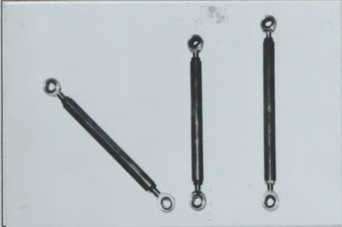
PHOTO No T9 Reinforced front stabilizer with linkage TYPE A
