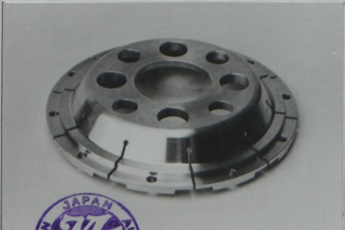
PHOTO No V3 Front brake mounting bell TYPE C
