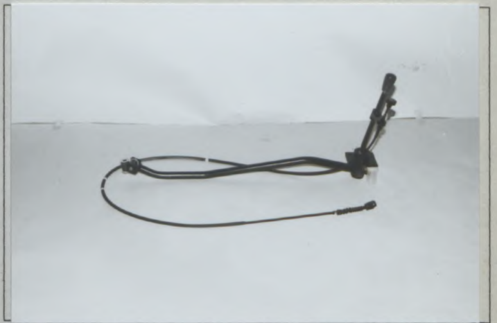
PHOTO No S6 Additional gearbox control linkage, TYPE C
