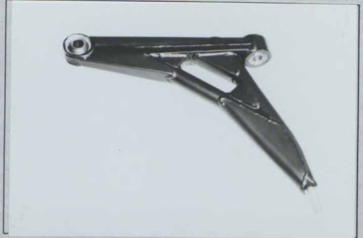
PHOTO No T8 Reinforced transeverse link TYPE D
