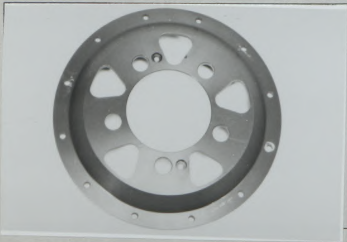
PHOTO No VW11 Front and/or Rear brake mounting bell, TYPE D
