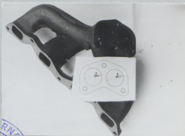
Q. exhaust manifold
