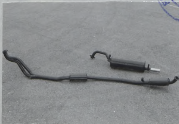
I. silencer + exhaust pipes after exhaust manifold.
