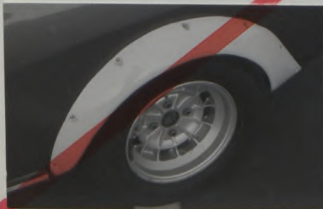
Photo. Rear wing extension
