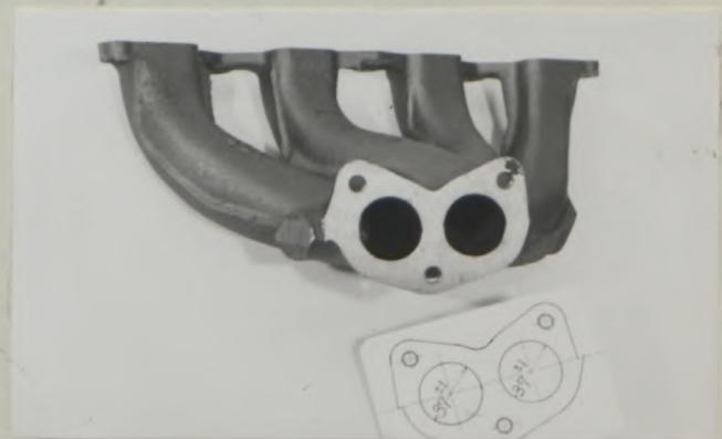
Q, Exhaust manifold
