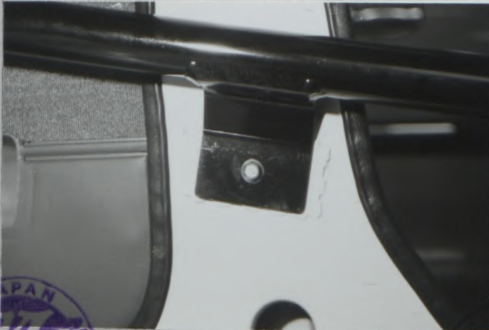
E) Diagonal strut to pillar
