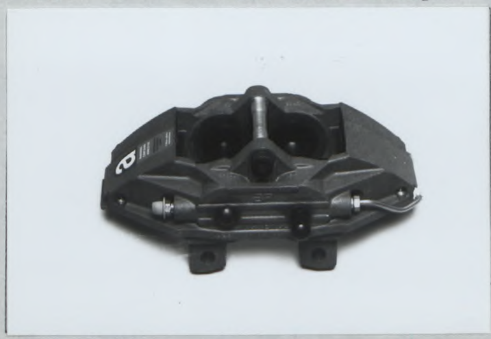
Photo V1 Front disc brake caliper
