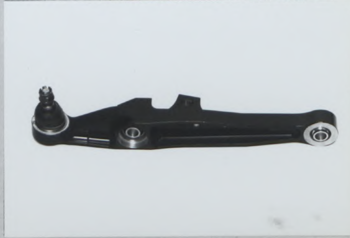
Photo T4 Reinforced front lower arm
