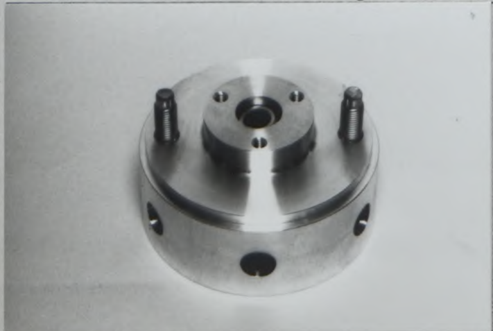
Photo T5 Reinforced front damper mount
