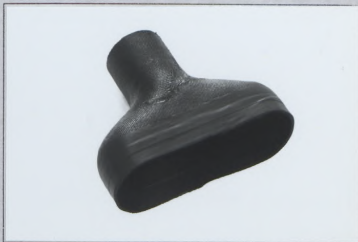
photoU2 Front brake cooling air intake
