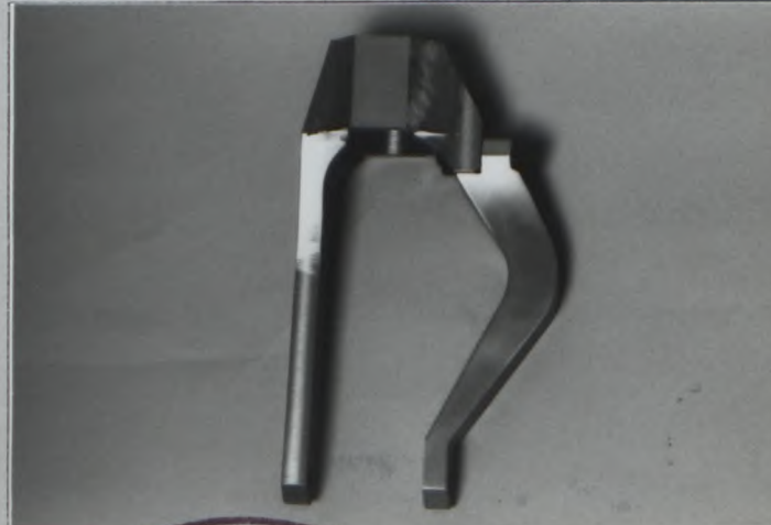
Photo T6 Reinforced front damper fork
