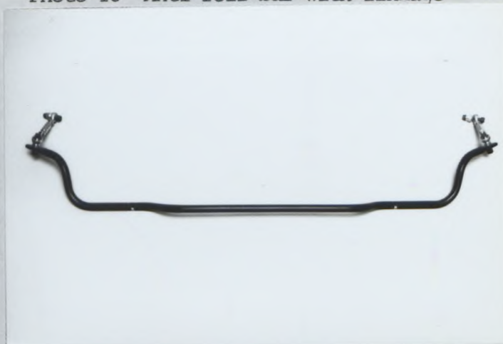
Photo T8 Adjustable front Anti-roll bar with linkage
