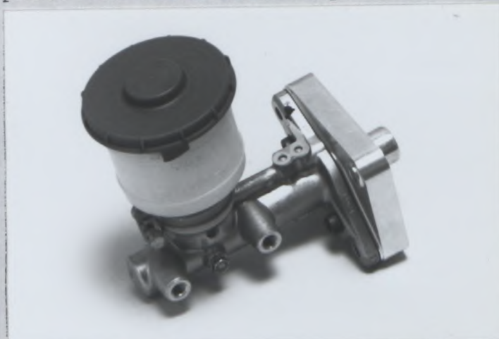
photo V1: Brake master cylinder
