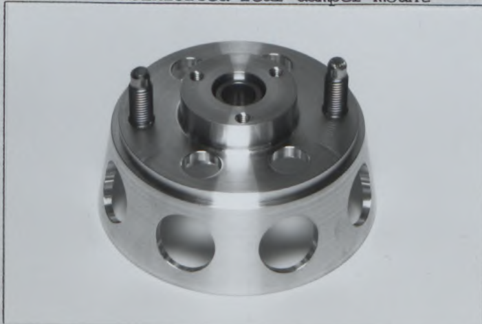
Photo T3 Reinforced rear damper mount
