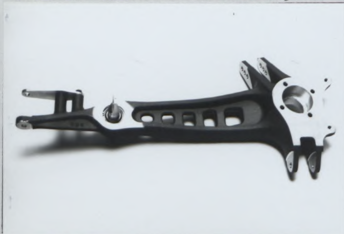
Photo T13 Reinforced rear trailing arm
