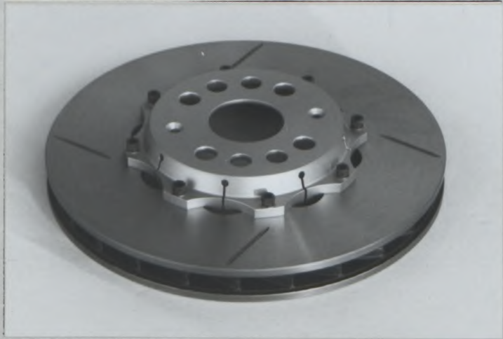
Photo V3 Front brake disc (Groove type) Photo W1 Rear disc brake caliper
