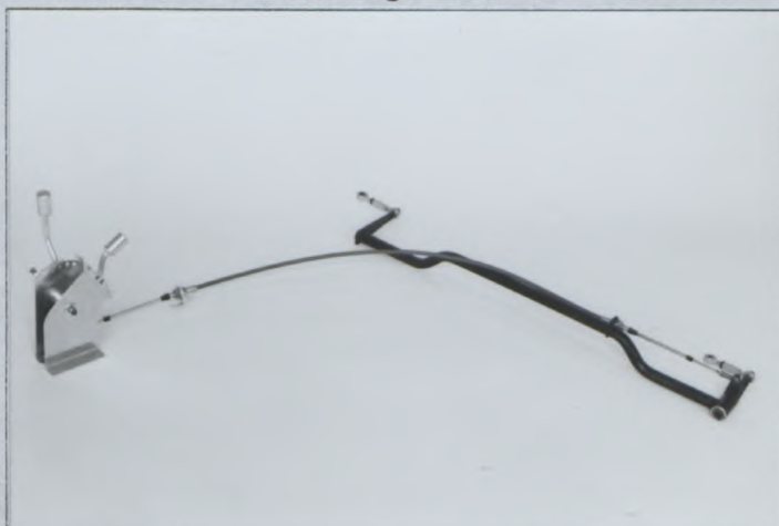
Photo T2 Adjustable front anti-roll bar with linkage
