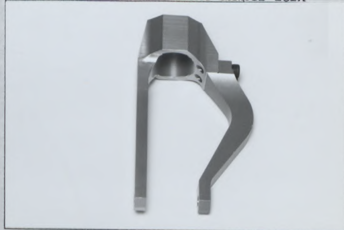
Photo T2 Reinforced front damper fork
