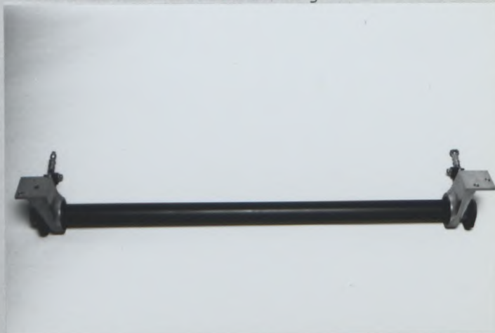
Photo T16 Adjustable rear anti-roll bar with linkage
