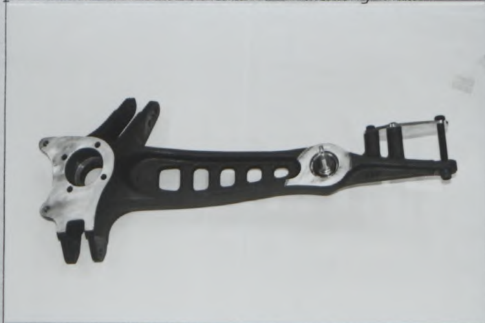
photo T3 Reinforced rear trailing arm
