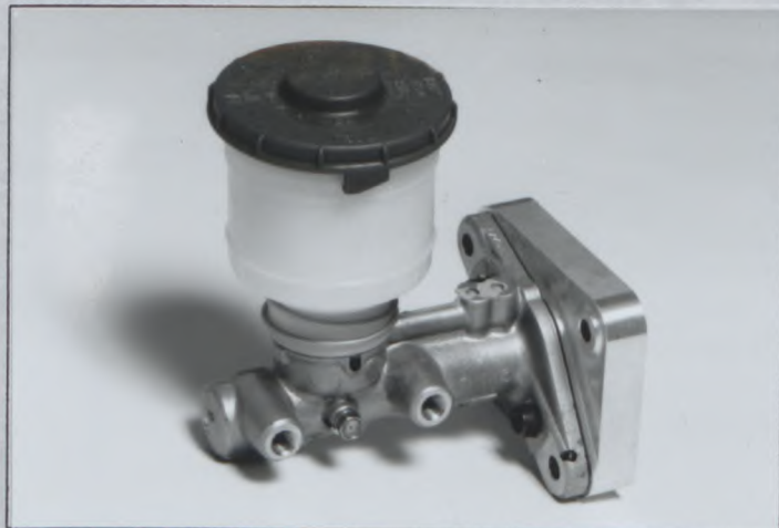
Photo V1 Brake master cylinder
