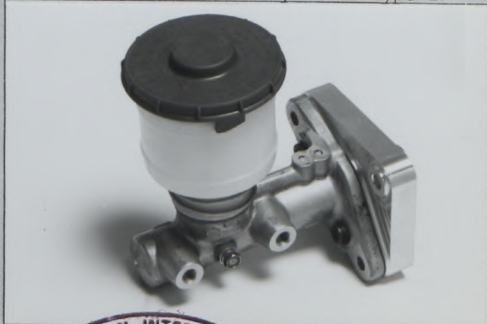
Photo V2 Brake master cylinder type 2
