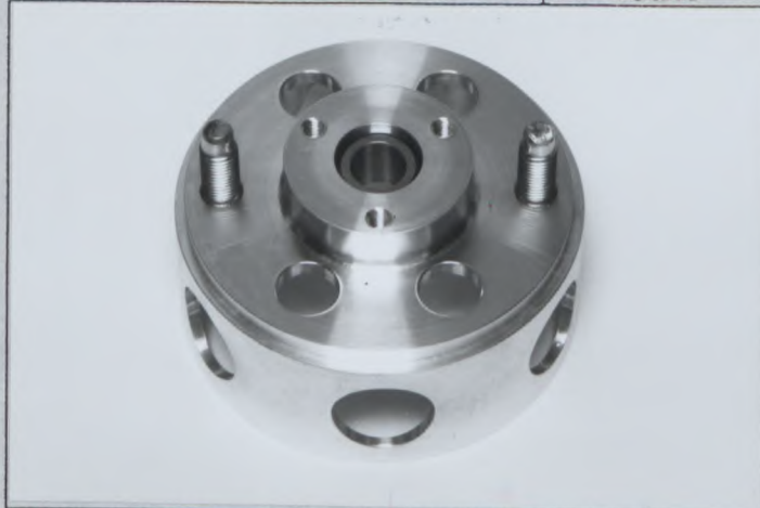
Photo T1 Reinforced front damper mount
