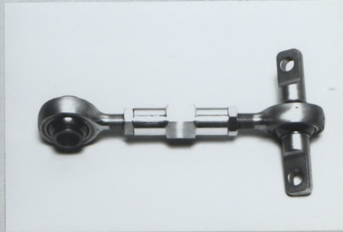
Photo T10 Reinforced rear upper arm
