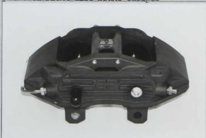
photo U1 Front disc brake caliper
