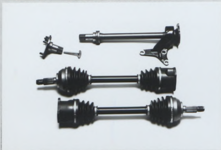
Photo T1 Reinforced drive shaft
