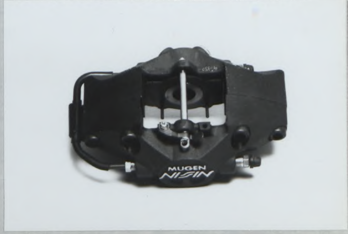
Photo V3 Front brake disc (Groove type) Photo W1 Rear disc brake caliper
