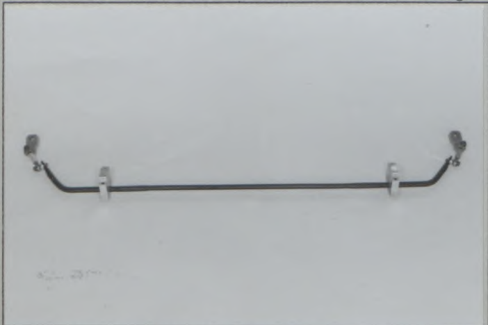
Photo T5 anti-roll bar with linkage
