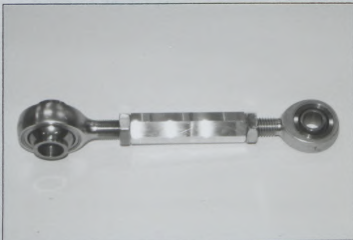
photoT8 Reinforced rear compensator arm
