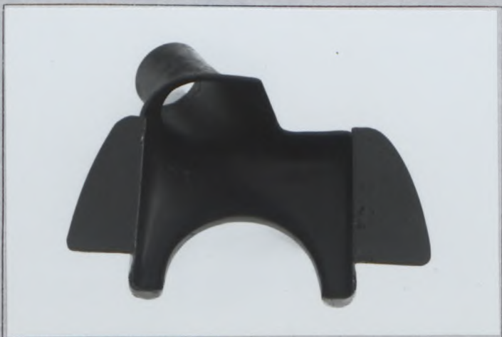
photoU3 Front brake cooling air outlet
