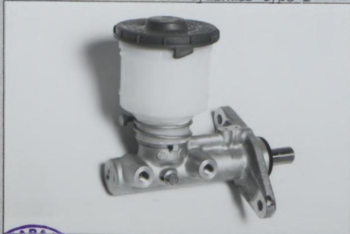
Photo V1 Brake master cylinder type 1
