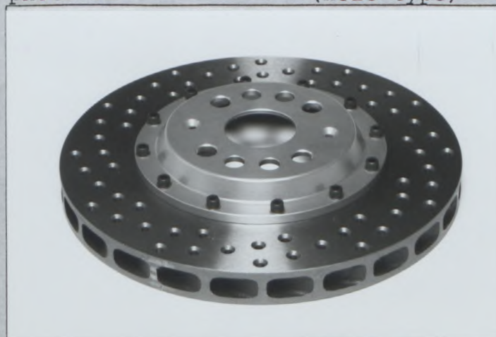
photo V5 Front brake disc type 2 (Hole type)
