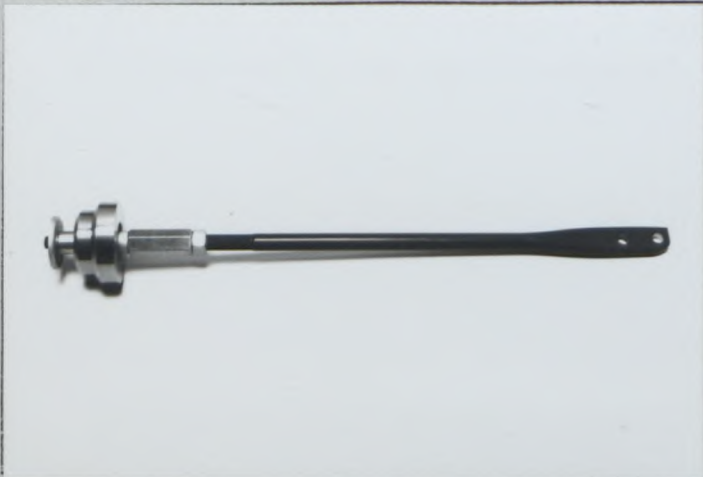
Photo T3 Reinforced front radius arm
