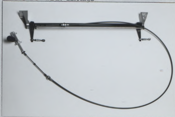
Photo T4 Adjustable rear anti-roll bar with linkage
