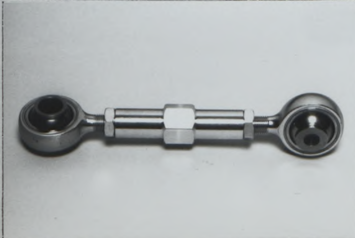
Photo T11 Reinforced rear Compensator arm
