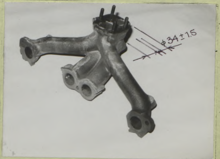
J) Izduvna grana Exhaust manifold
