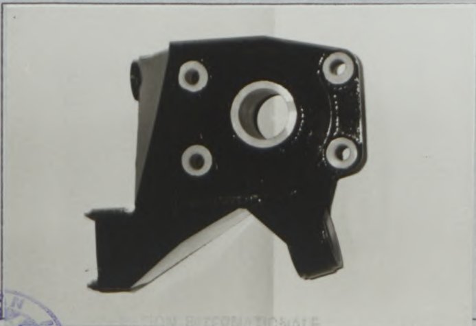
PHOTO No U1 REINFORCED REAR KNUCKLE TYPE E
