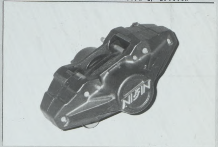
PHOTO No VW2 FRONT AND/OR REAR BRAKE CALIPER TYPE 2, 2PISTON
