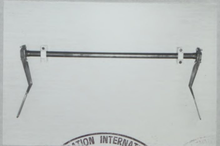
PHOTO No TU6 FRONT AND/OR REAR REINFORCED STABILIZER TYPE A
