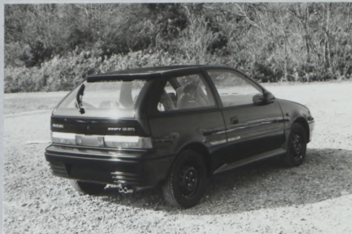
Photo B ADOPTION OF NEW DESIGNED REAR BUMPER INCLUDED REAR COMBNATION LAMP
