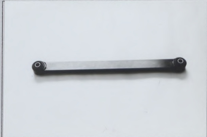
PHOTO U1 REINFORCED REAR ARM
