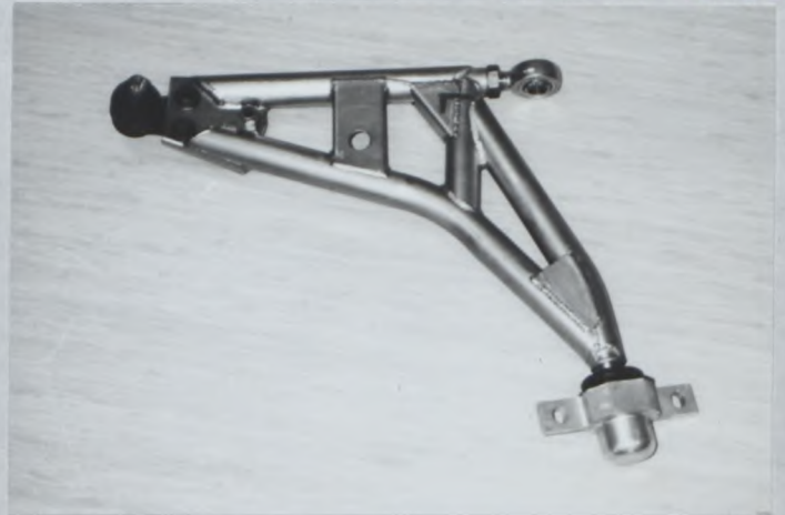
PHOTO No T1 REINFORCED FRONT ARM MA-128 VO-11/9
