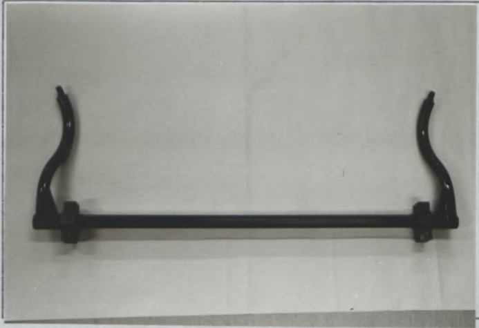
PHOTO No T5 REINFORCED FRONT STABILIZER TYPE C
