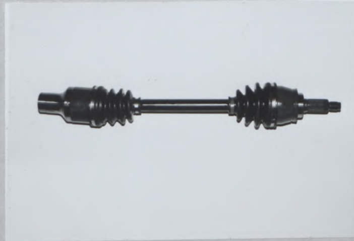
PhotoZ1 Reinforced drive shaft RH
