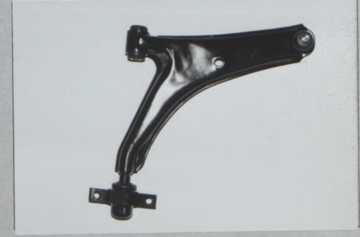
PhotoT3 Reinforced front suspension arm
