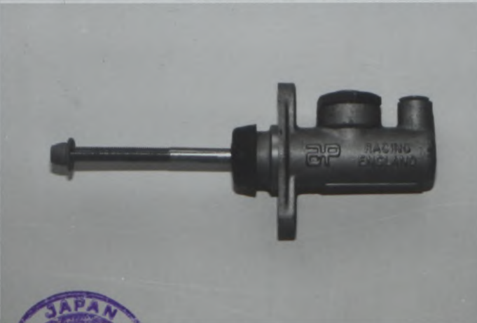
PHOTO No VW1 BRAKE AND/OR CLUTCH MASTER CYLINDER
