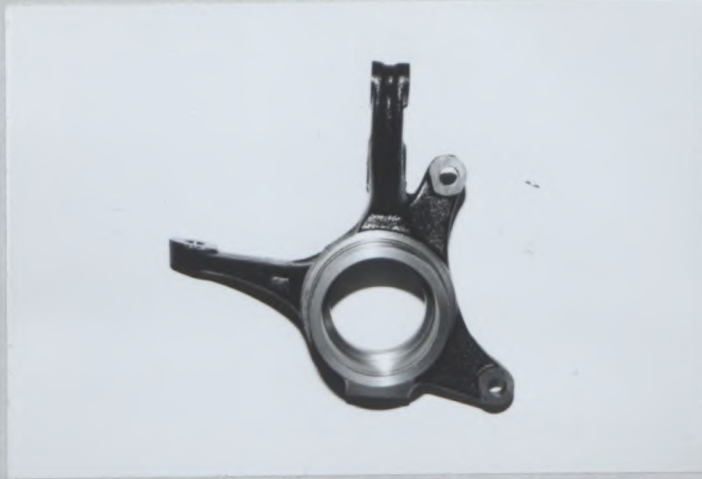
PhotoT1 Reinforced front knuckle
