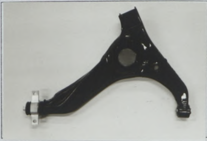
PHOTO No U3 REINFORCED REAR ARM TYPE C
