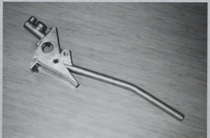
PHOTO No VW6 REINFORCED PARKING BRAKE
