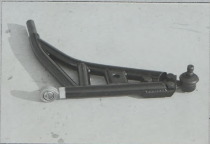
Photo T5 LOWER ARM, REINFORCED
