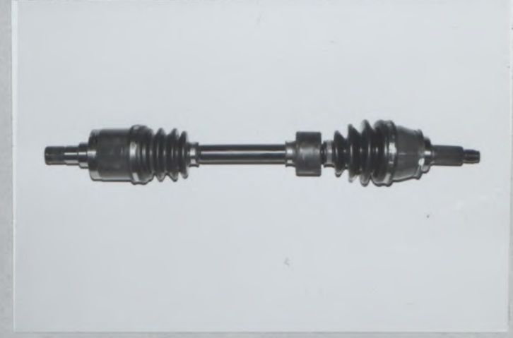
PhotoZ2 Reinforced drive shaft LH
