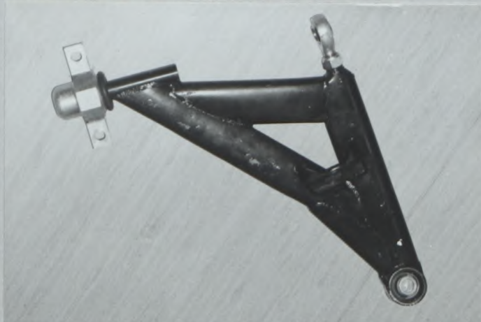
PHOTO No T3 REINFORCED FRONT ARM TYPE C
