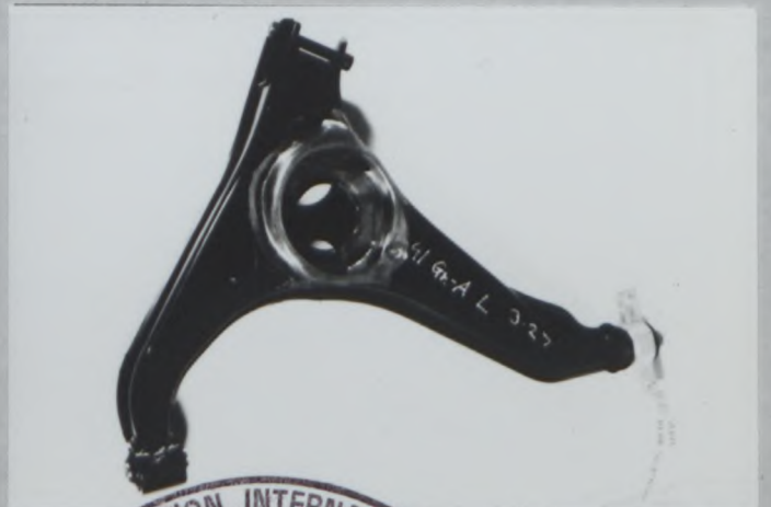
PHOTO No U1 REINFORCED REAR ARM
