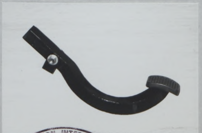
PHOTO No Z1 REINFORCED CLUTCH PEDAL TYPE A
