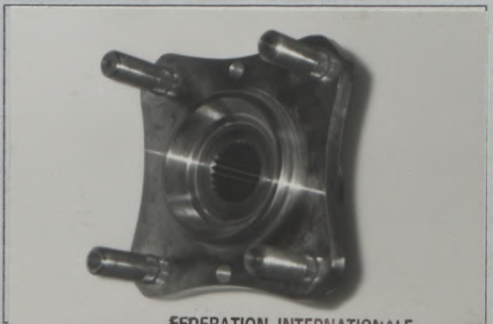
PHOTO No T4 REINFORCED FRONT WHEEL HUB TYPE C
