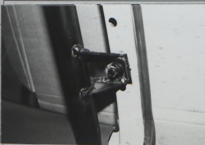
MAIN HOOP TO PILLAR
