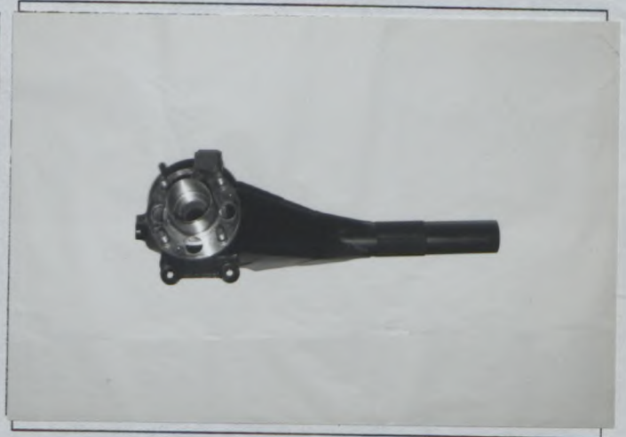
PHOTO T3 REINFORCED UPRIGHT
