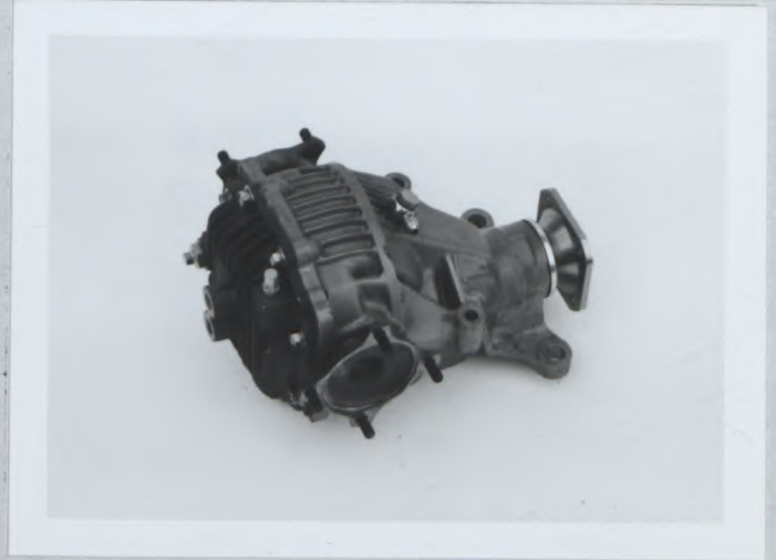
PHOTO 28 REINFORCED DIFFERENTIAL HOUSING
