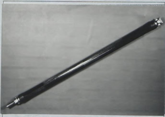
PHOTO Z8 REINFORCED PROPELLER SHAFT
