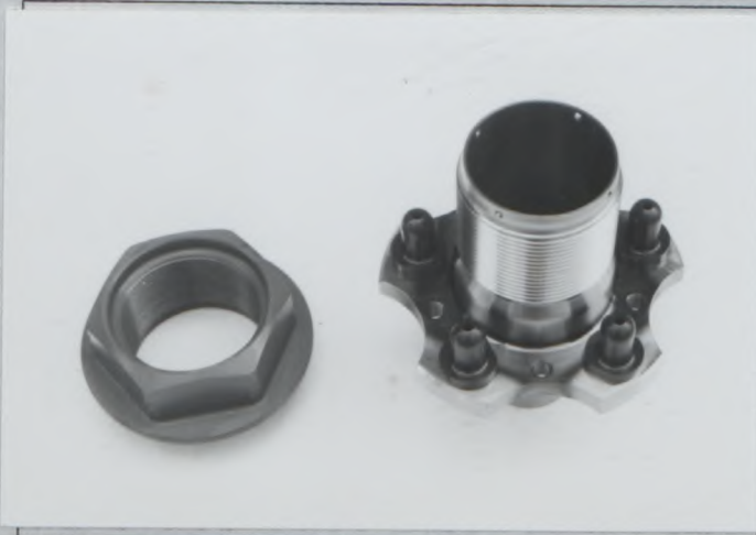
PHOTO T3 CENTRAL WHEEL BOLTING SYSTEM
