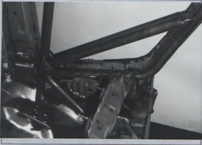
FRONT HOOP TO PILLAR (LEFT HAND SIDE)
