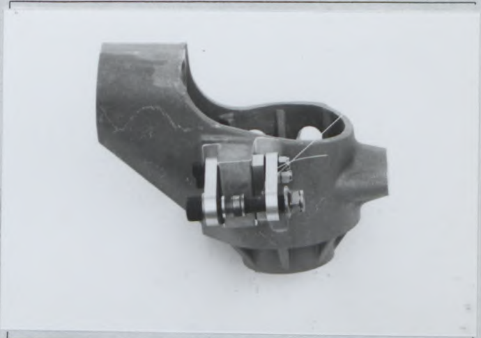
PHOTO T8 REINFORCED KNUCKLE
