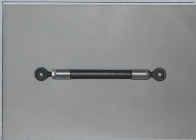
PHOTO U4 REINFORCED TRACK CONTROL ARM, TYPE B
