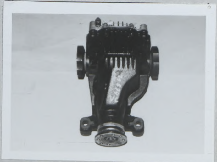
PHOTO Z6 REAR DIFFERENTIAL CASING
