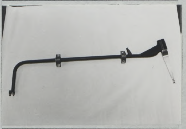
PHOTO U1 REAR ADJUSTABLE STABILISER ASSEMBLY WITH ANCHORAGE POINTS MODIFIED
