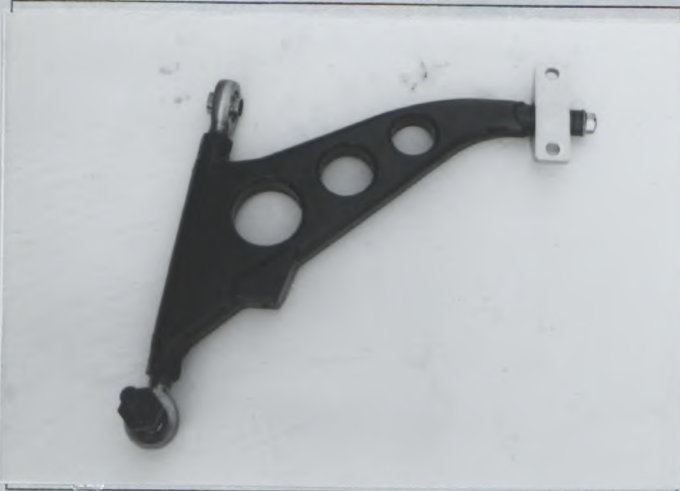
PHOTO T1 REINFORCED LOWER ARM
