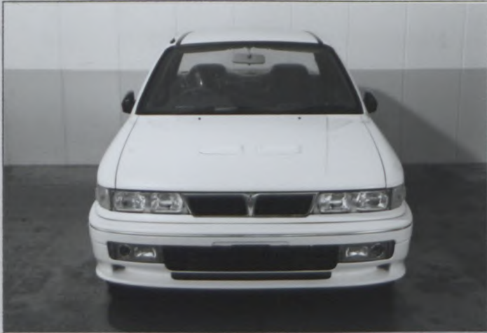
Air inlet added on front bumper and A1 air outlet added on hood
