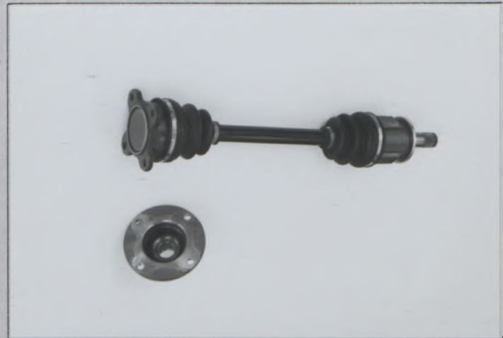
Z Reinforced rear drive shaft and companion flange
