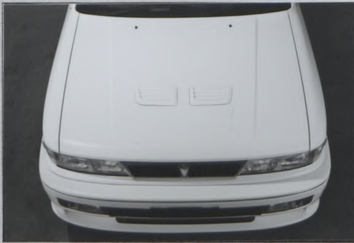
A3 Air outlet added on hood
