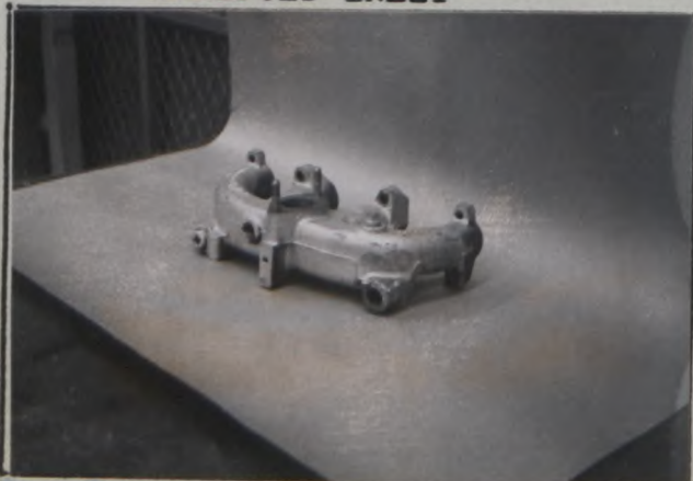
P MANIFOLD INLET
