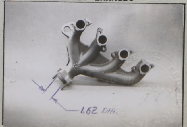
Q MANIFOLD EXHAUST
