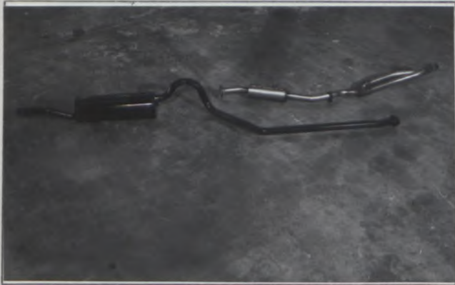
I, Silencer + exhaust pipes after exhaust manifold.
