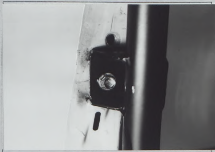
MAIN HOOP TO PILLAR
