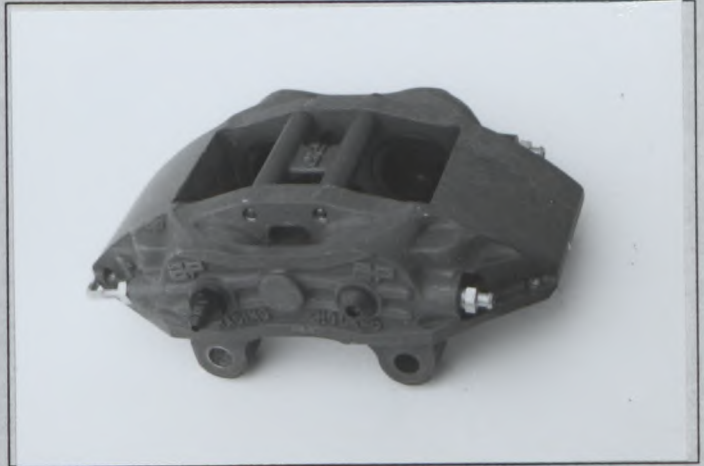
Photo W2 Rear brake caliper TYPE B
