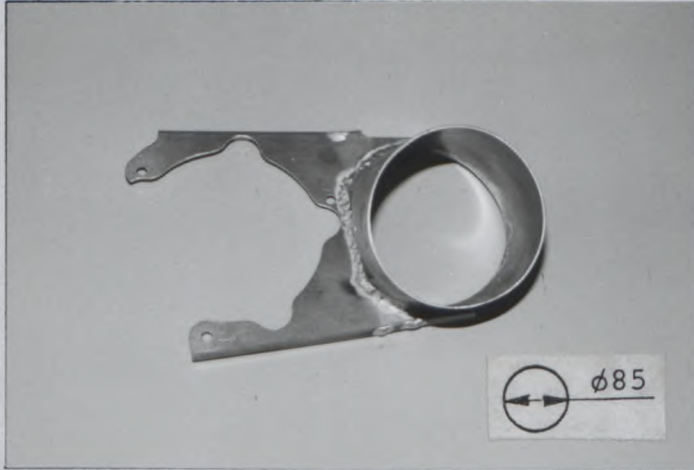
Photo Z6 Rear brake air duct TYPE A
