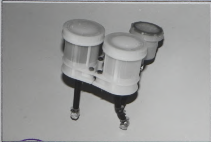
Photo Z10 Twin brake master cylinder reservoir tank TYPE A
