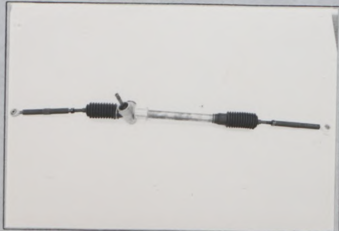
Photo Z4 Heavy duty steering gear box and side rods
