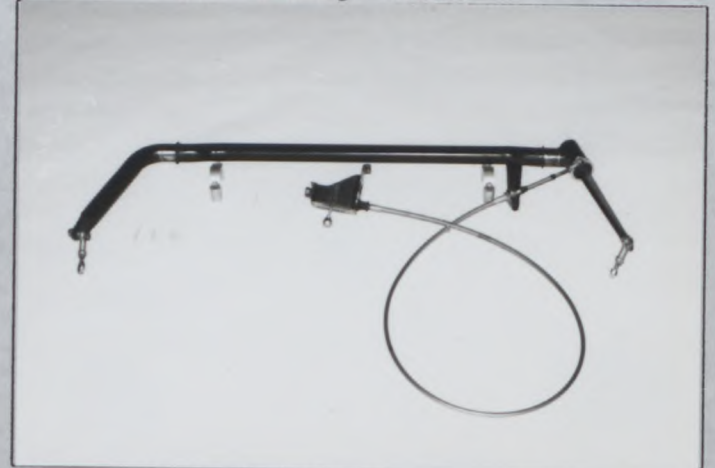
Photo Z5 Heavy duty steering arm TYPE B and spacer
