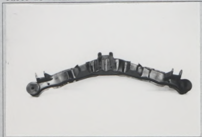
Photo Z3 Reinforced rear suspension member
