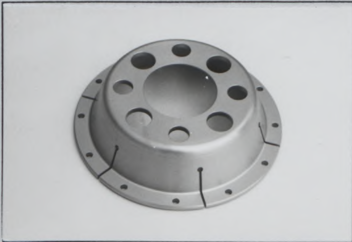
Photo Z2 Rear brake mounting bell TYPE D
