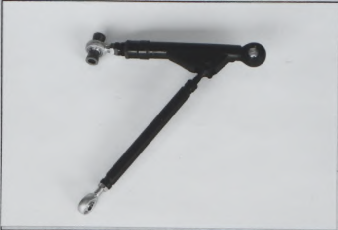
Photo T3 Alternative transverse link and tension rod
