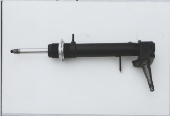
Photo T3 Adjustable front stabilizer with linkage TYPE E
