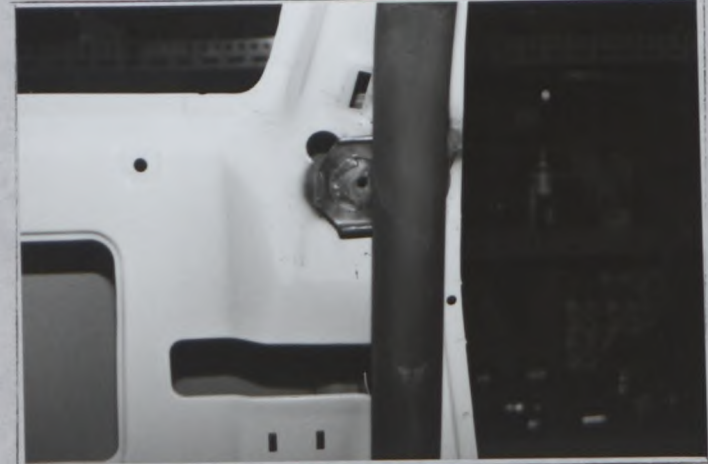
Main hoop to pillar
