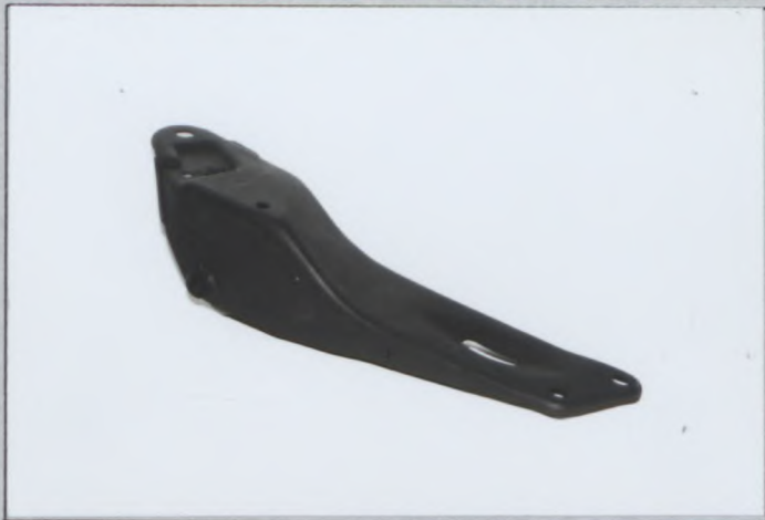
Photo T2 Reinforced tension rod bracket
