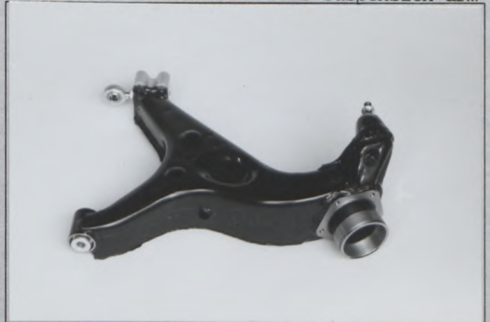
Photo U1 Reinforced rear suspension arm
