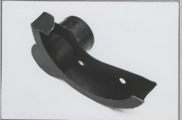
Photo Z11 Reinforced differential mounting bracket
