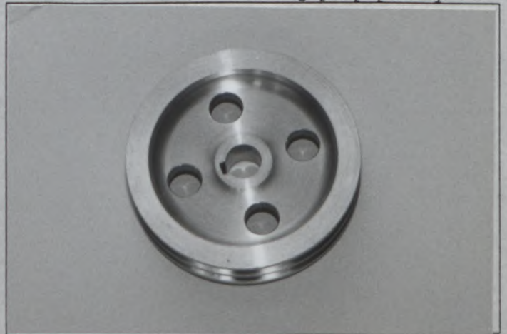
Photo Z5 Power steering pump pulley
