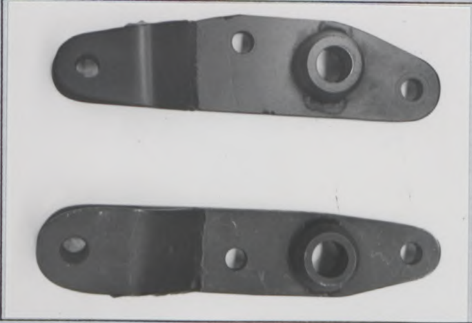
Photo Z6 Heavy duty steering arm TYPE C
