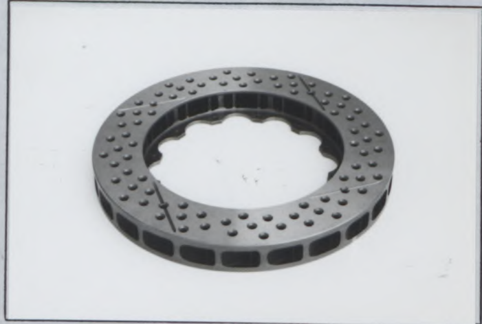
Photo V2 Front brake disc TYPE E
