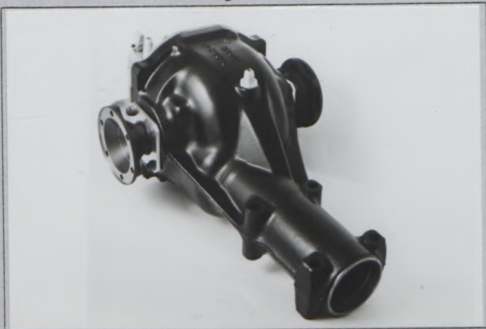
Photo Z5 Reinforced differential housing
