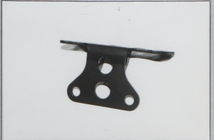
Photo Z11 Reinforced differential mounting bracket
