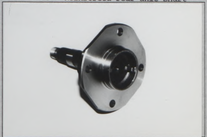
Photo U3 Reinforced rear axle shaft
