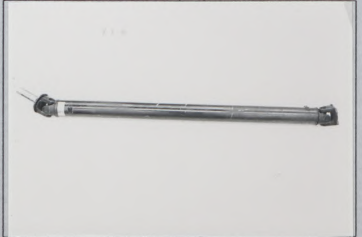
Photo Z1 Reinforced propeller shaft
