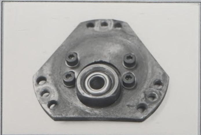
Photo T5 Reinforced front strut top mount TYPE B
