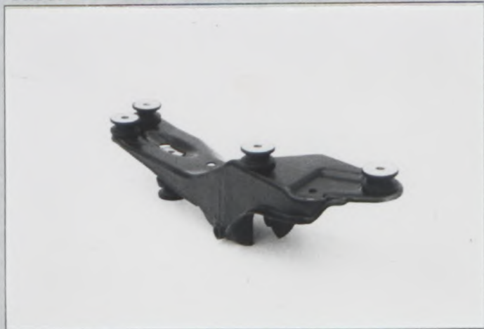
Photo Z3 Reinforced rear suspension member
