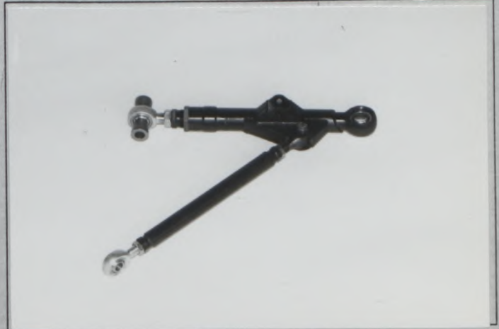
Photo T1 Alternative transverse link and tension rod
