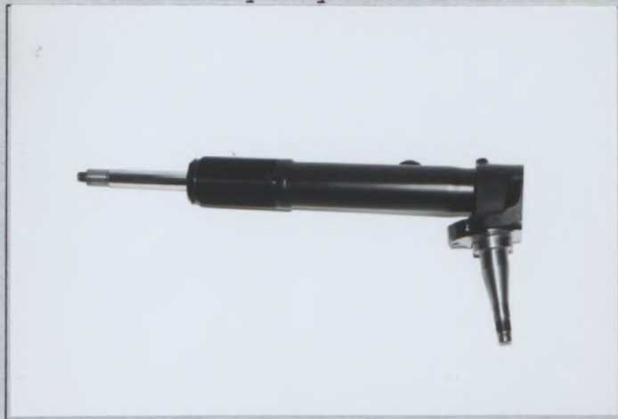
Photo T5 Adjustable front stabilizer with linkage TYPE A
