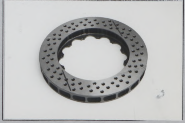
Photo W3 Rear brake disc TYPE E~H
