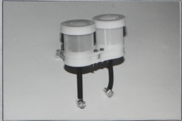
Photo Z11 Twin brake master cylinder reservoir tank TYPE B
