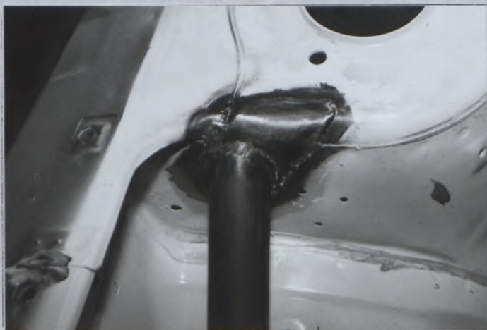
Front reinforcements to strut tower
