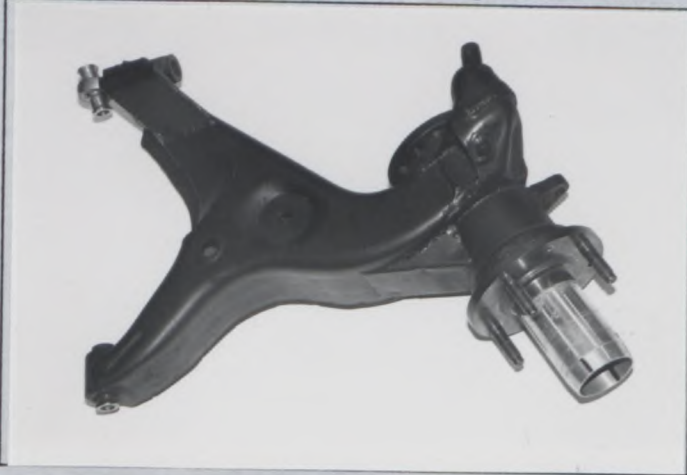
Photo U1 Heavy duty rear suspension arm
