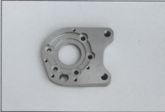
Photo T8 Front brake caliper mounting bracket
