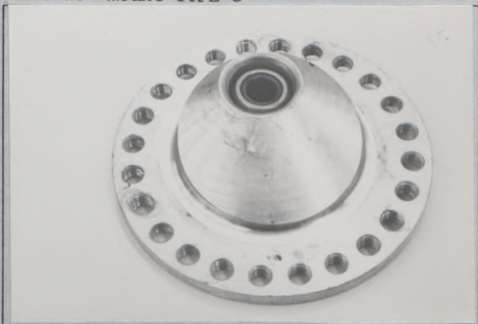
Photo T6 Reinforced front strut top mount TYPE C
