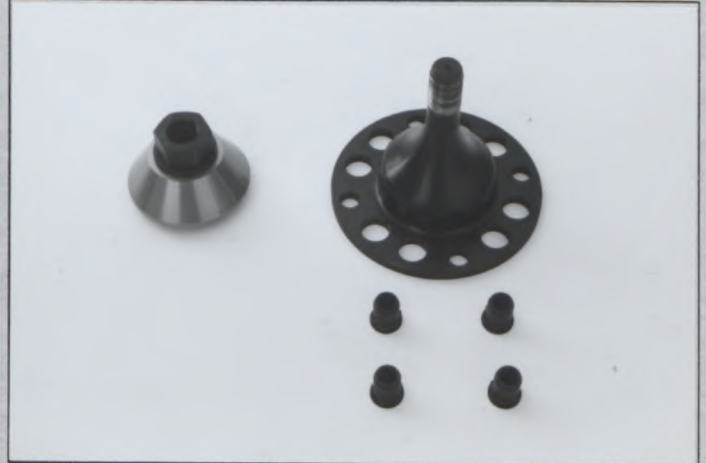
Photo Z17 Center fixing wheel hub and lock nuts
