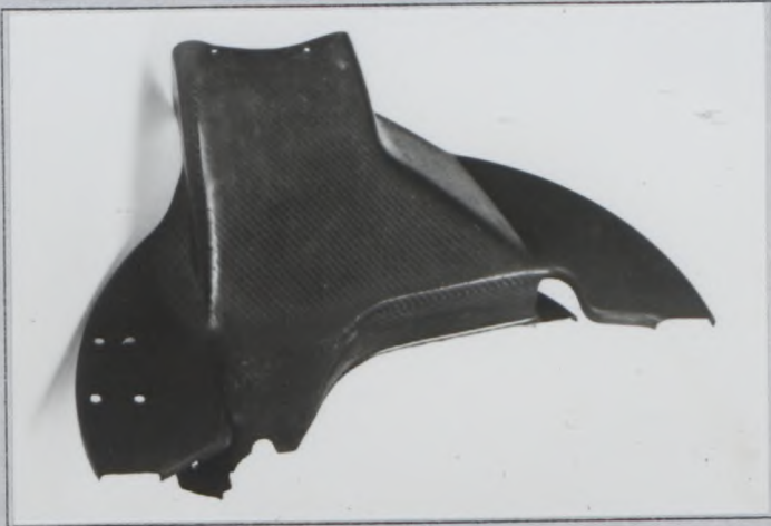
Photo Z5 Reinforced differential housing
