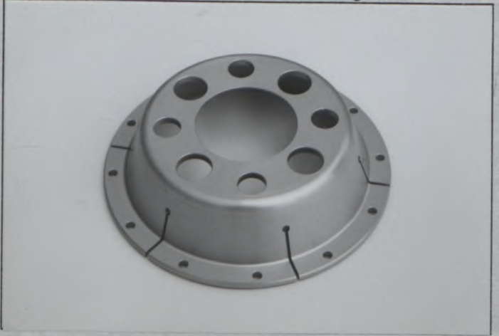
Photo Z10 Rear brake mounting bell TYPE A
