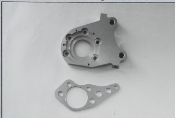
Photo T4 Front brake caliper mounting bracket and stay
