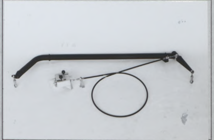
Photo U7 Adjustable rear stabilizer with linkage TYPE B
