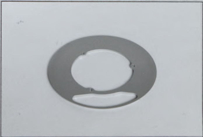
Photo Z15 Rear brake dust shield TYPE B
