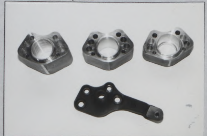
Photo Z5 Heavy duty steering arm TYPE B and spacer
