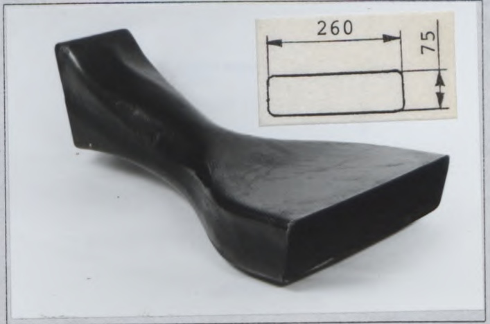
Photo Z2 Front brake air duct
