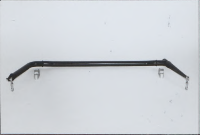
Photo U6 Adjustable rear stabilizer with linkage TYPE A
