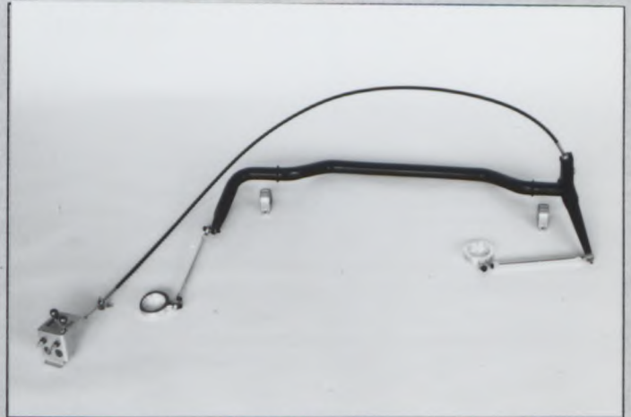
Photo T2 Adjustable front stabilizer with linkage TYPE D
