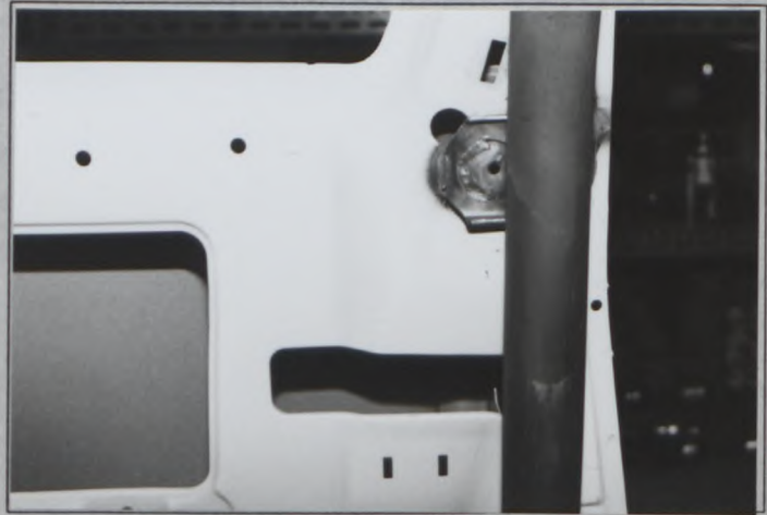
Main hoop to pillar
