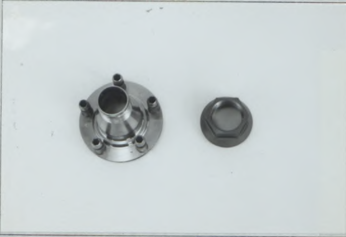
Z1 Central knock off drive system for front & rear wheels
