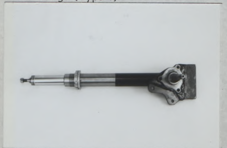
T6 Reinforced front strut and brake caliper mountings (Type 3)
