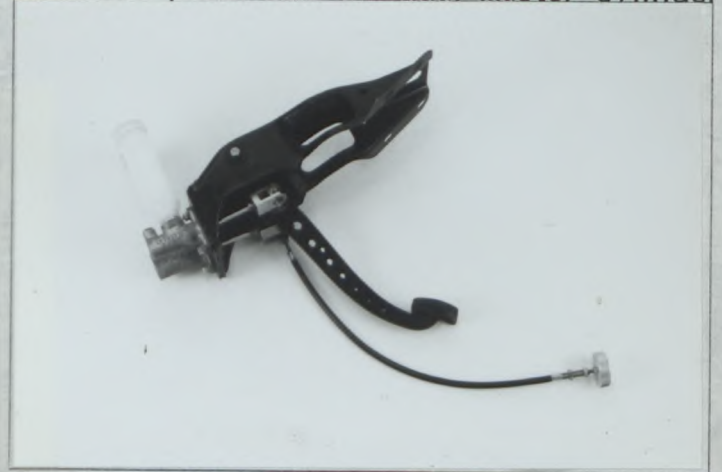
Z2 Brake pedal box for dual master cylinder
