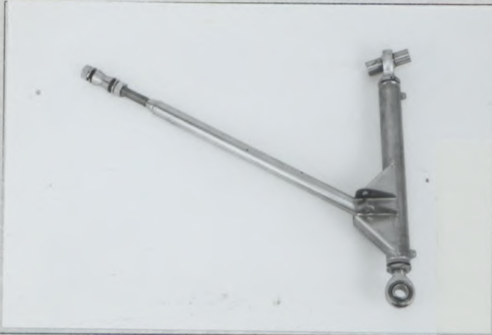
T1 Reinforced front control arm and caster-rod (Type 1)
