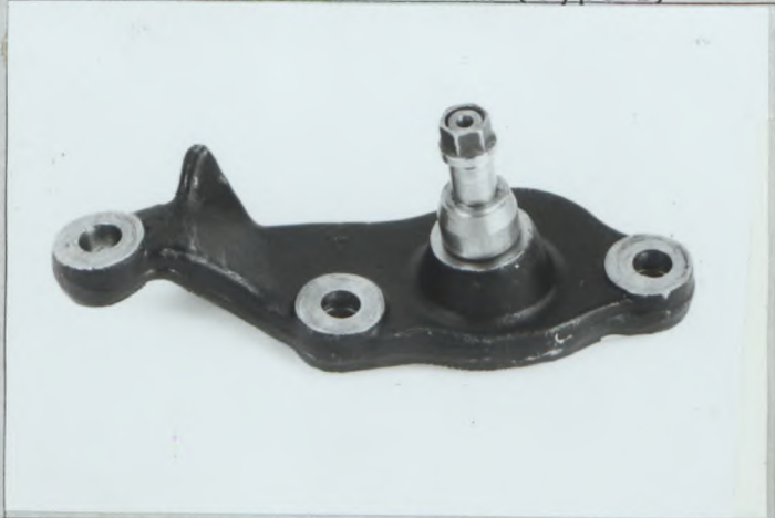
Z19 Reinforced knuckle arm (Type 2)
