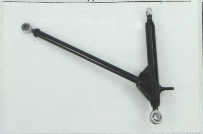
T2. Reinforced front control arm and caster-rod (Type 2)
