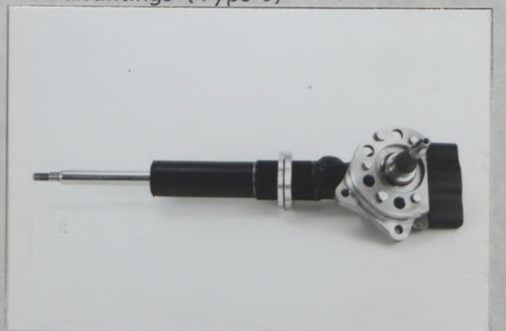
T6 Reinforced front strut and brake caliper mountings (Type 3)
