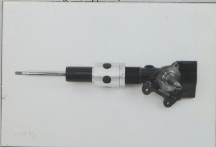
T5 Reinforced front strut and brake caliper mountings (Type 2)
