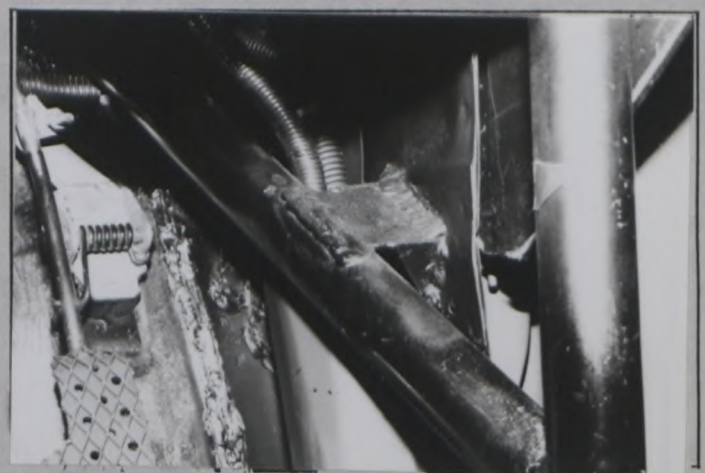
Front reinforcement to dash side
