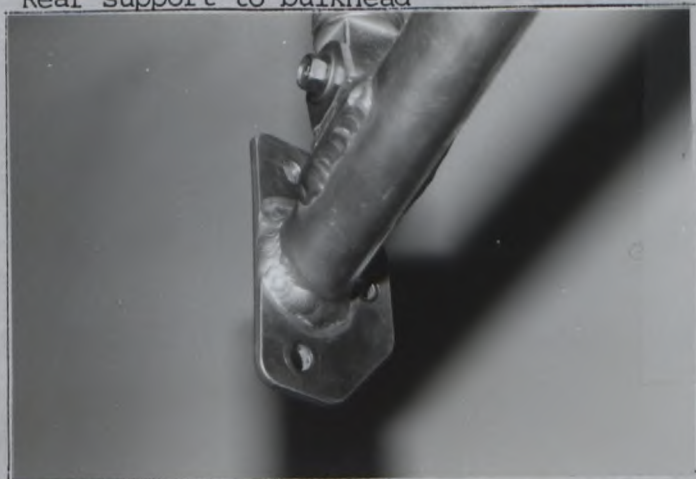
Rear support to bulkhead
