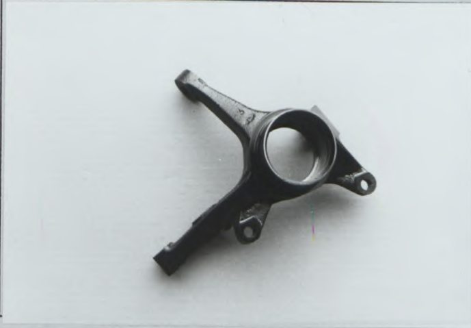
PhotoT1 Reinforced front knuckle
