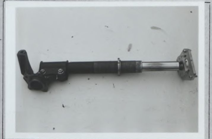
Photo U3 Reinforced rear strut
