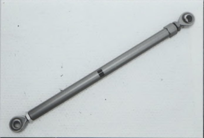
Photo U2 Reinforced rear strut rod
