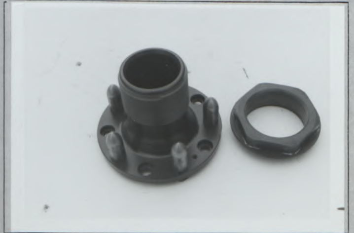
Photo Z3 Center fixing wheel hub
