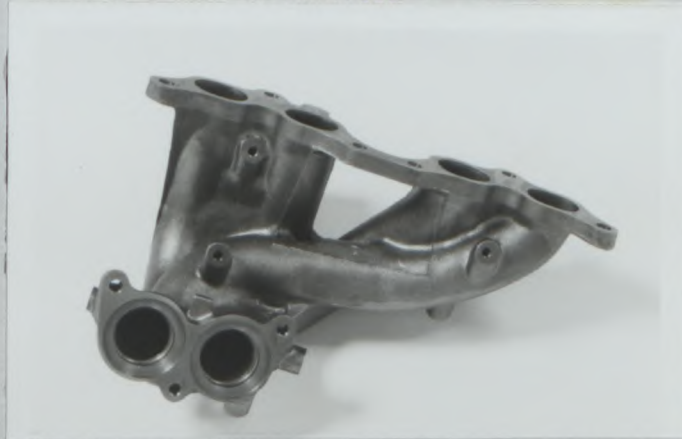
PHOTO J1 EXHAUST MANIFOLD
