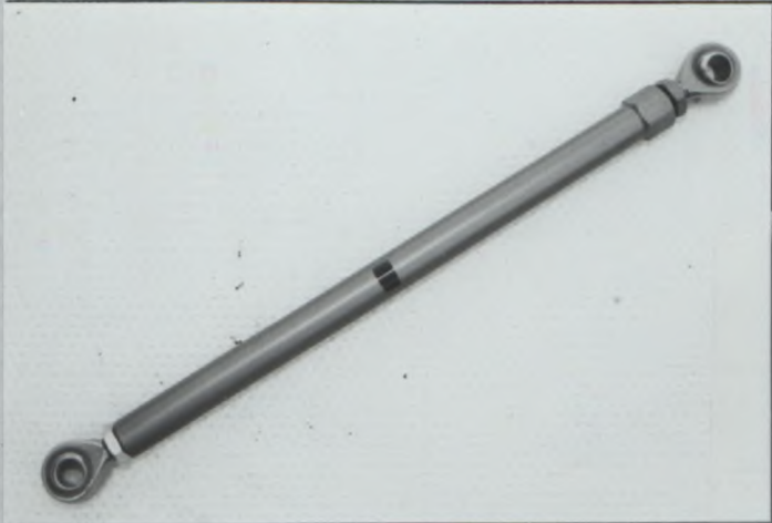
Photo U2 Reinforced rear strut rod
