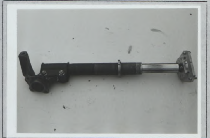
Photo U3 Reinforced rear strut
