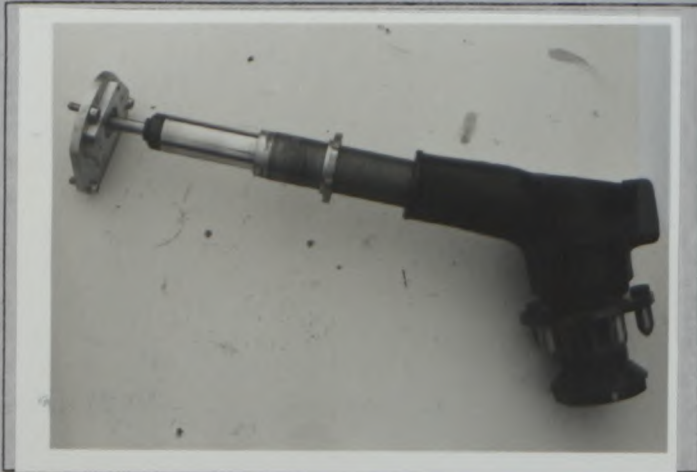
Photo T2 Reinforced front strut
