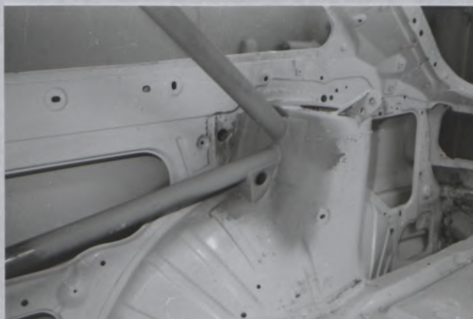
Longitudinal strut to rear strut tower
