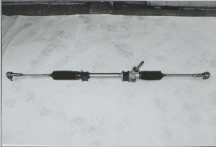
Photo Z3 Steering gear box
