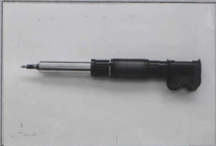
Photo T3 Reinforced front strut
