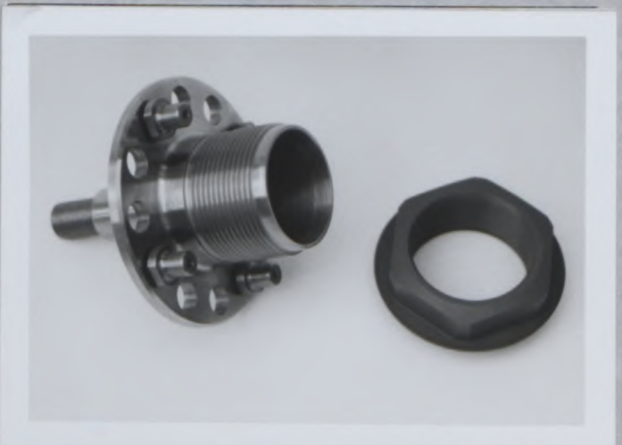
PHOTO U3 CENTRAL WHEEL BOLTING SYSTEM
