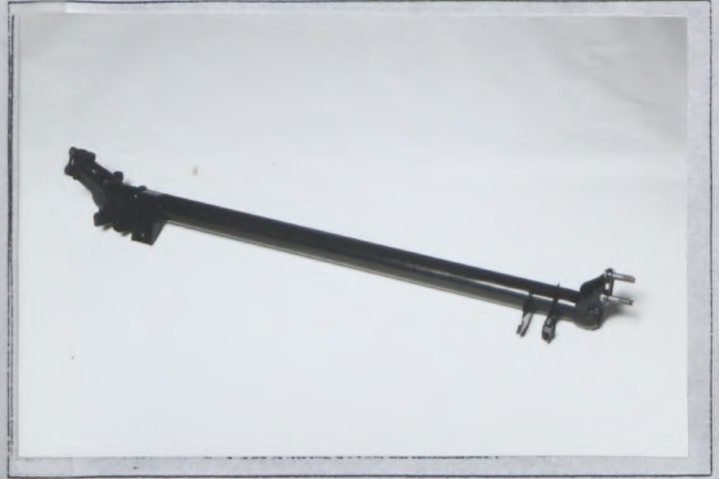
photo T4 Reinforced rear axle beam
