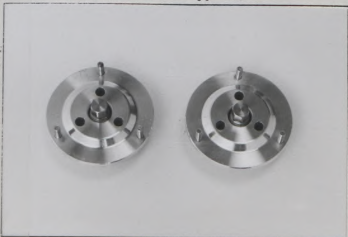
T4 Alternative adjustable top mounting for front strut (Type A)
