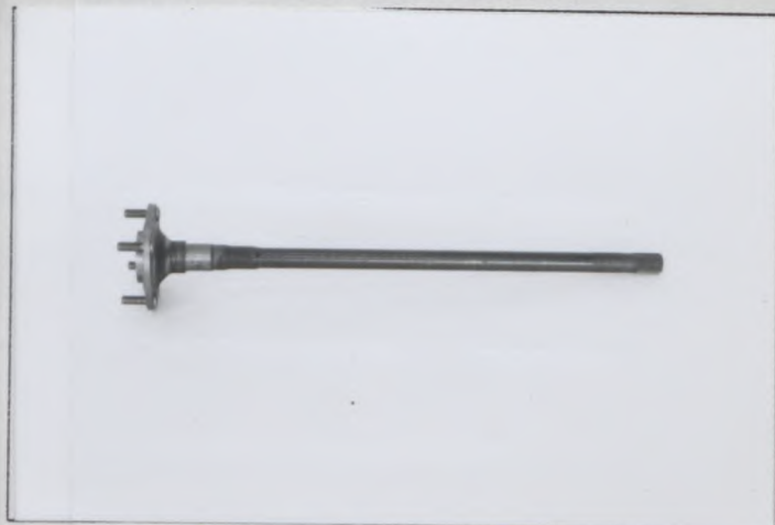
Z5 Reinforced rear axle shaft
