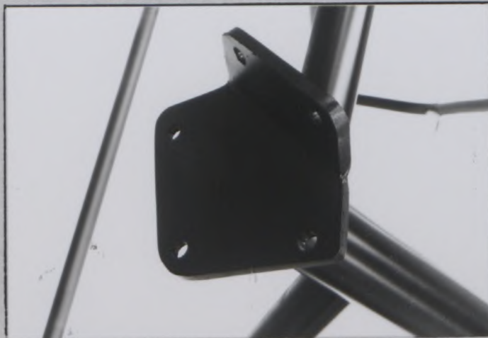
Rear support to bulkhead
