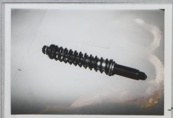
Alternative position of rear spring Photo U5 and shock absorber
