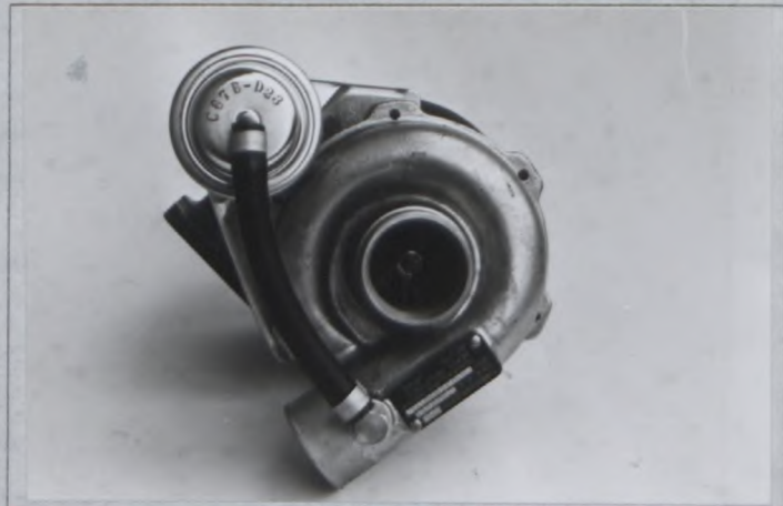
O) Valve and by-pass installation of compressor 過給圧調整装置
