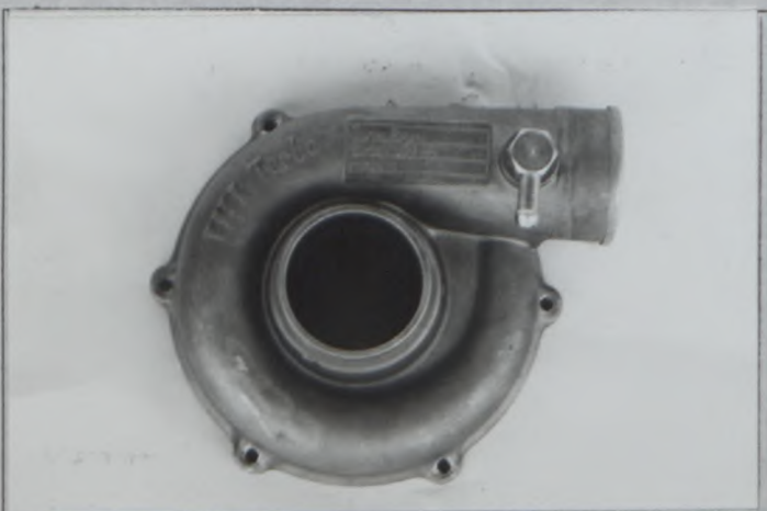
Q) Inlet between the turbocompressor and the atmosphere 空気取入口
