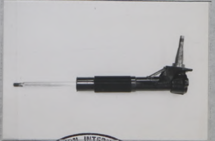
Photo T4 Reinforced front strut
