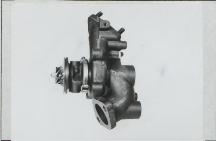
O) Valve and by-pass installation of compressor
