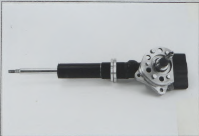
T3 Reinforced front strut and brake caliper mountings (Type 3)
