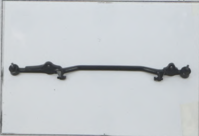
Z1 Reinforced steering cross shaft (Type 1)
