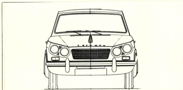
Track to be checked with wheels at 0° camber.
