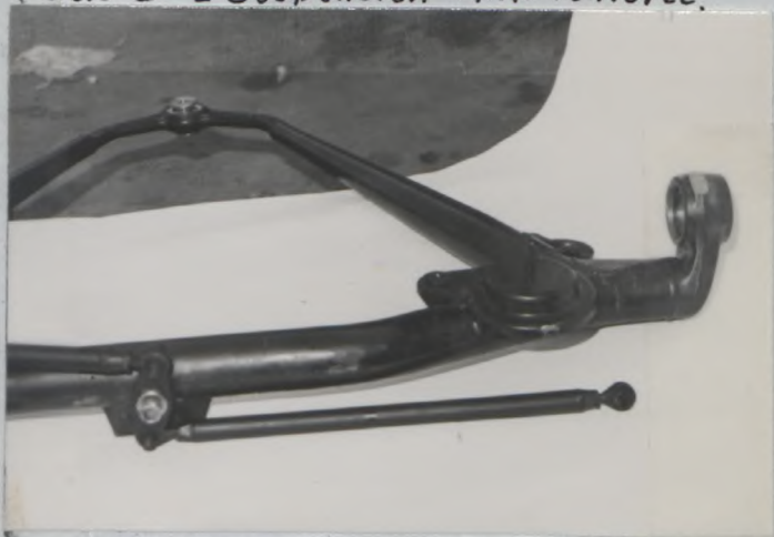
Photo U' = Suspension A.R. renforcé
