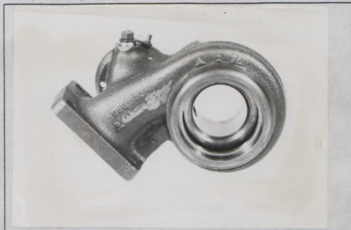
P) Exhaust between the manifold and the turbocompressor 排気ガス入口
