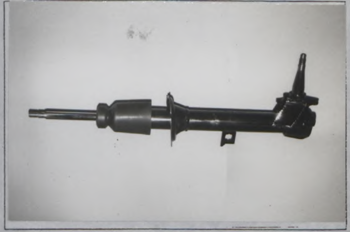
Photo T 2 Reinforced front strut
