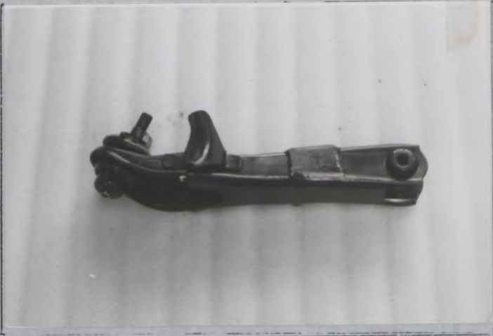
Photo T 1 Reinforced front lower arm
