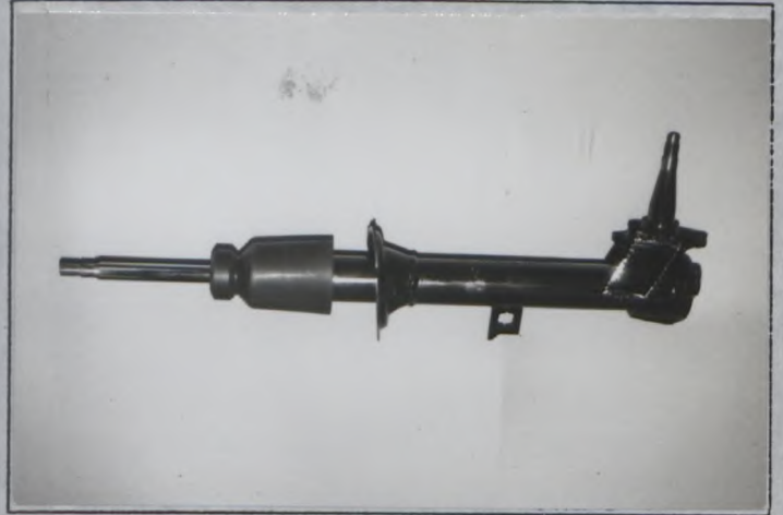
Photo T 2 Reinforced front strut
