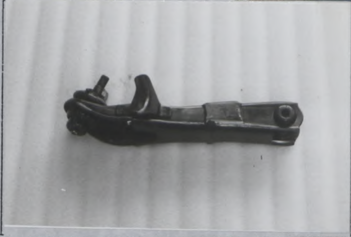
Photo T 1 Reinforced front lower arm
