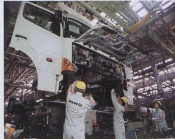
A cab takes its place on a chassis. | キャブの搭載。
