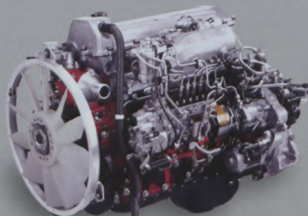
Euro 1 J08C Engine Displacement: 7.961 l, 6-cylinder in-line Max output: 155kW (210PS)/2,900rpm (JIS GROSS)
