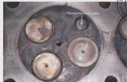
Konstantdrossel : lifting of a small valve in the combustion-chamber during the compression stroke of the engine
