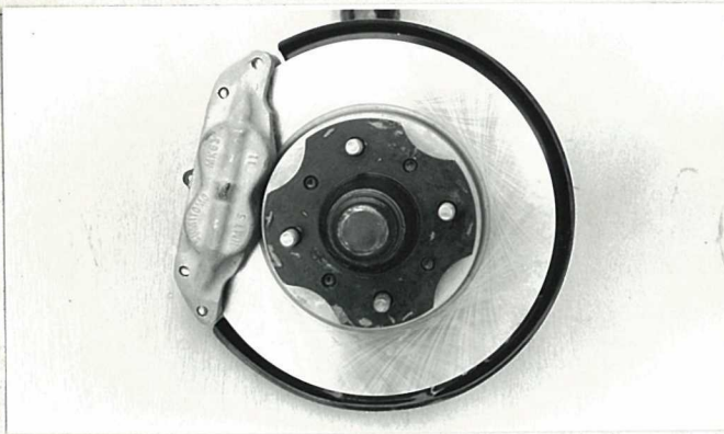
Photograph F, Front brake disc with caliper
