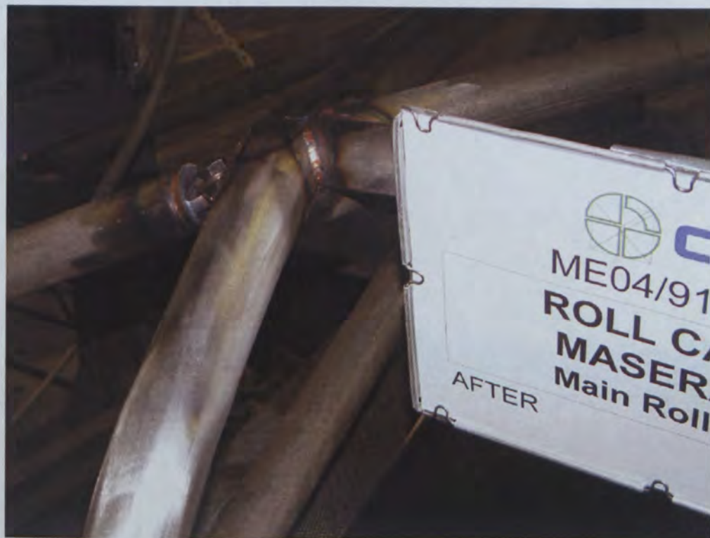
Picture five: Main roll bar after the test
