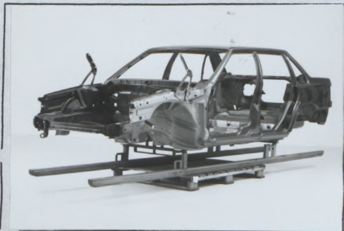
A9) Coque vue de 3/4 avant, sans portes, capots, etc. Bodyshell seen from 3/4 front without doors, lids, etc.
