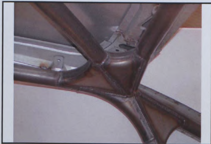
PHOTO N° 9 front roll bar with longitudinal member to roof reinforcement diagonal member (left side)
