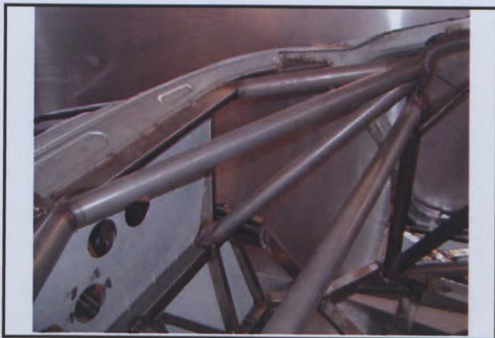
PHOTO N° 6 front roll bar reinforcing members to chassis
