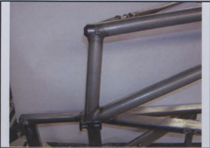
PHOTO N° 14 backstay fixation to chassis
