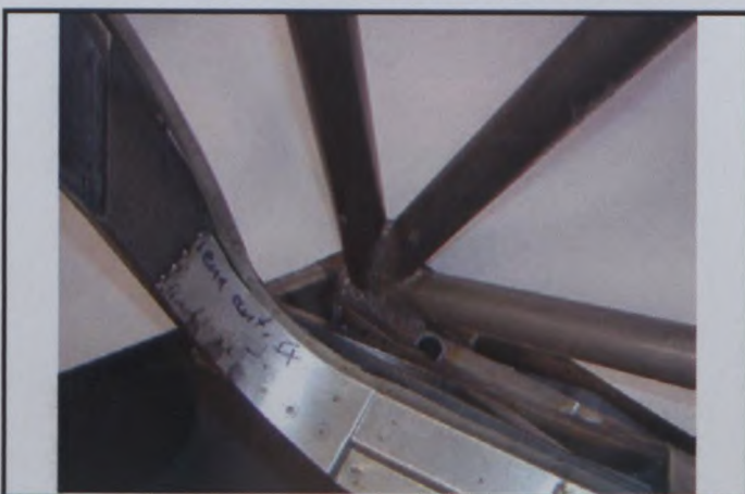
PHOTO N° 5 Front roll bar fixation to chassis
