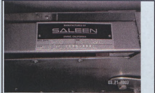
Plate Shown For All Chassis Built After 6-2002 Plate Info Contains MFG Date, Chassis ID #, & Saleen Part #
