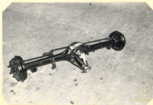
Rear axle complete (without wheels).
