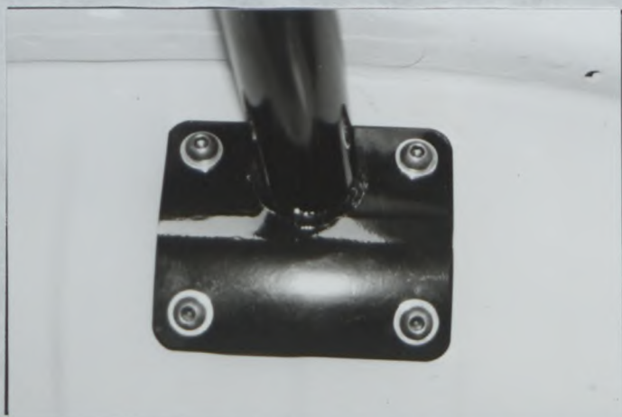
PHOTO N° 8. Rear support to wheel house RH
