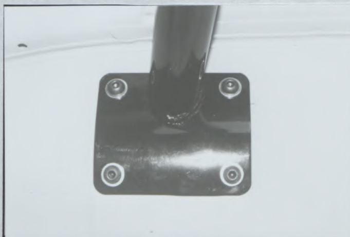
PHOTO N° 7. Rear support to wheel house LH
