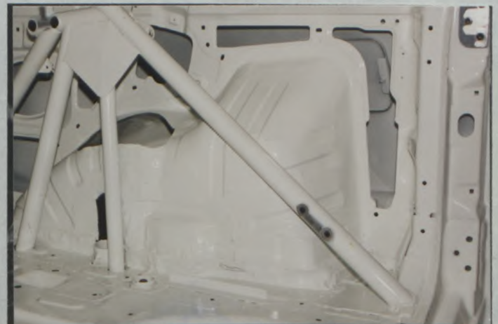
PHOTO N° 5 MAIN HOOP TO CENTER PILLAR
