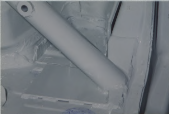
PHOTO N° 10 REAR SUPPORT BAR TO FLOOR
