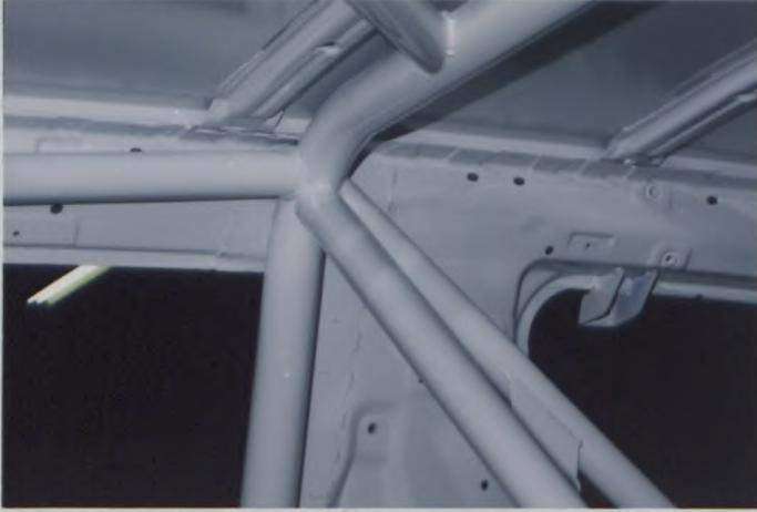
PHOTO N° 6 MAIN HOOP TO ROOF
