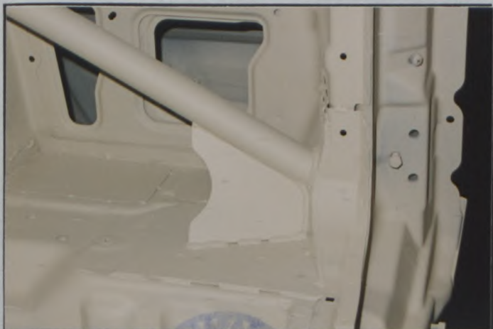
PHOTO N° 10 REAR SUPPORT BAR TO FLOOR
