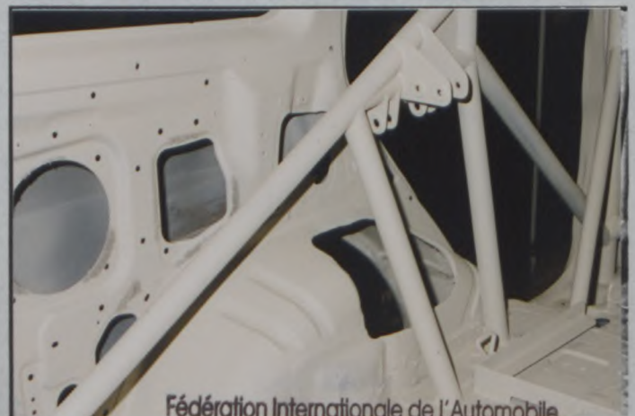
PHOTO N° 5 MAIN HOOP TO CENTER PILLAR
