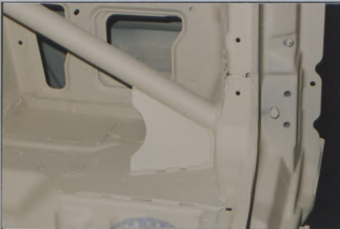
PHOTO N° 10 REAR SUPPORT BAR TO FLOOR
