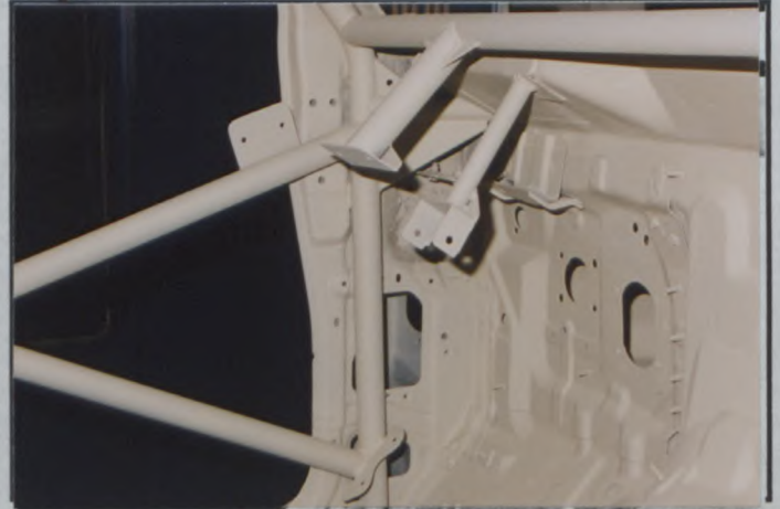
PHOTO N° 9 FRONT HOOP TO BULKHEAD
