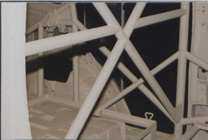
PHOTO N° 16 SEAT BELT BARS ON DIAGONAL
