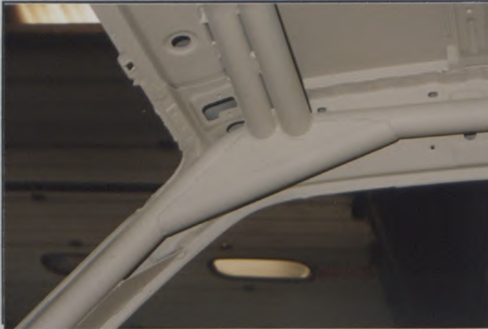
PHOTO N° 8 FRONT HOOP TO ROOF
