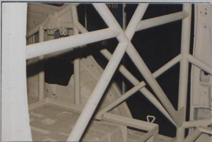
PHOTO N° 16 SEAT BELT BARS ON DIAGONAL
