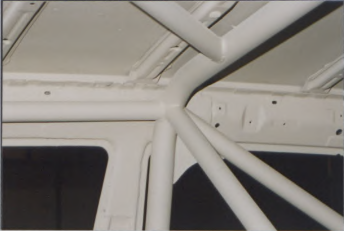
PHOTO N° 6 MAIN HOOP TO ROOF
