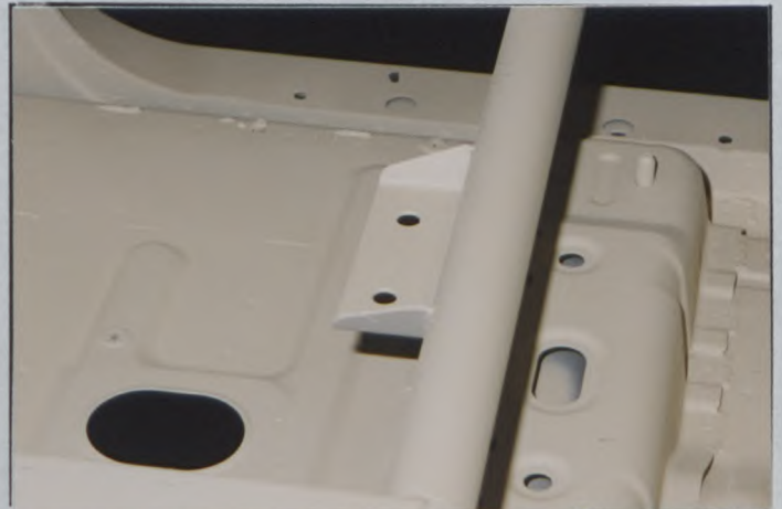
PHOTO N° 15 SEAT BELT BRACKET
