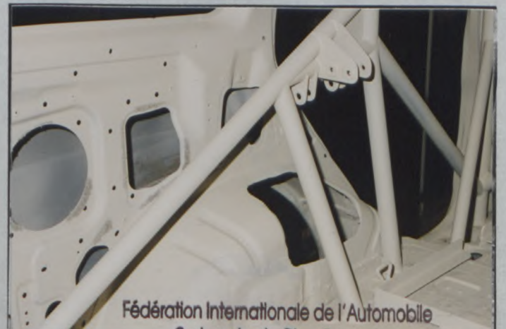
PHOTO N° 5 MAIN HOOP TO CENTER PILLAR
