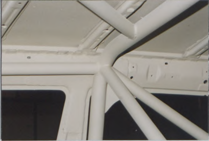
PHOTO N° 6 MAIN HOOP TO ROOF
