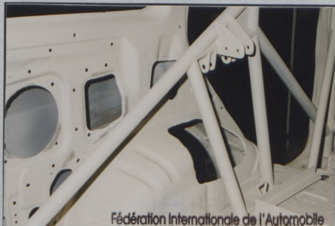
PHOTO N° 5 MAIN HOOP TO CENTER PILLAR
