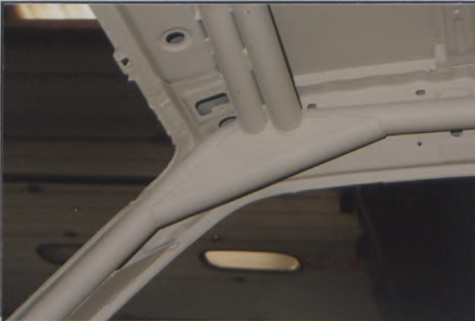
PHOTO N° 8 FRONT HOOP TO ROOF
